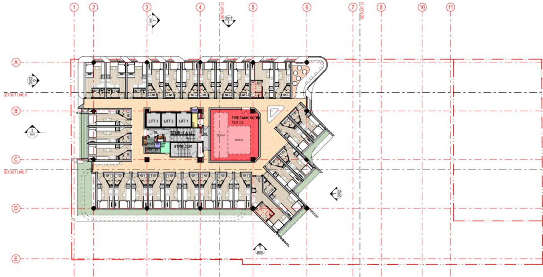
Figure 6.7: General arrangement Level 3 Source: fjcstudio 2026
