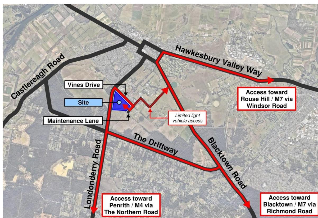
Figure 3.1: Recommended construction vehicle routes
