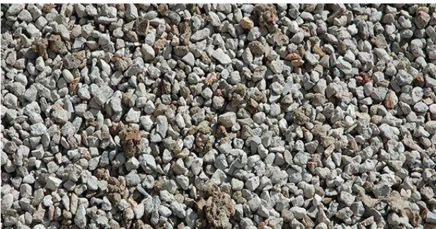
Recycled Crushed Materials for Paving (Paving Type 4)
