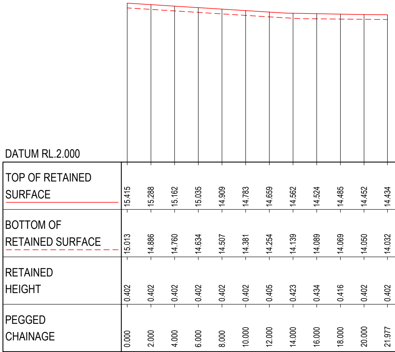
HOR : 1 IN 200 VERT: 1 IN 200 LONGITUDINAL SECTION - RW 07
