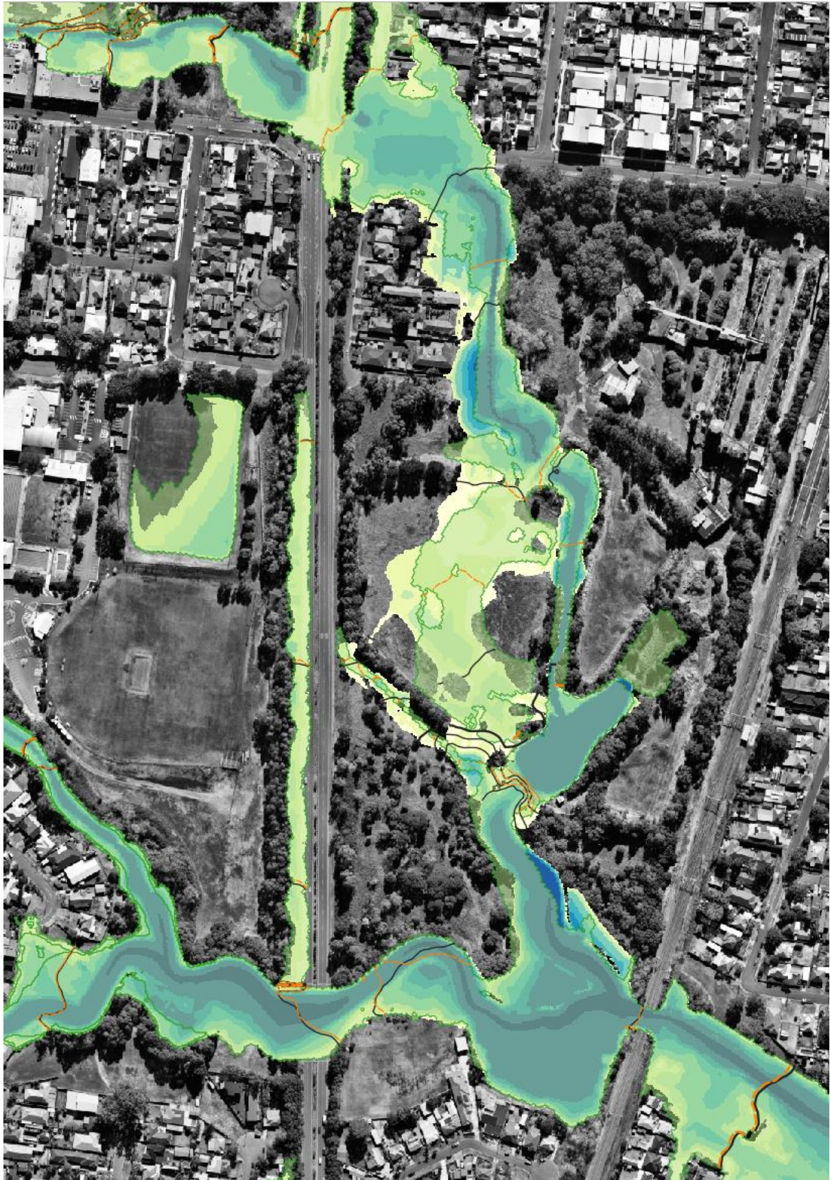
Figure 12: Published DFE depth and water level (black contours) and existing case extent (green) and water level (orange contours)
