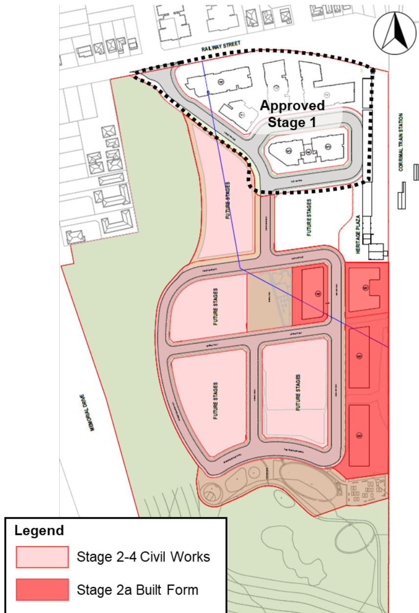
Figure 3.1: Stage 2-4 Civil Works Extent
