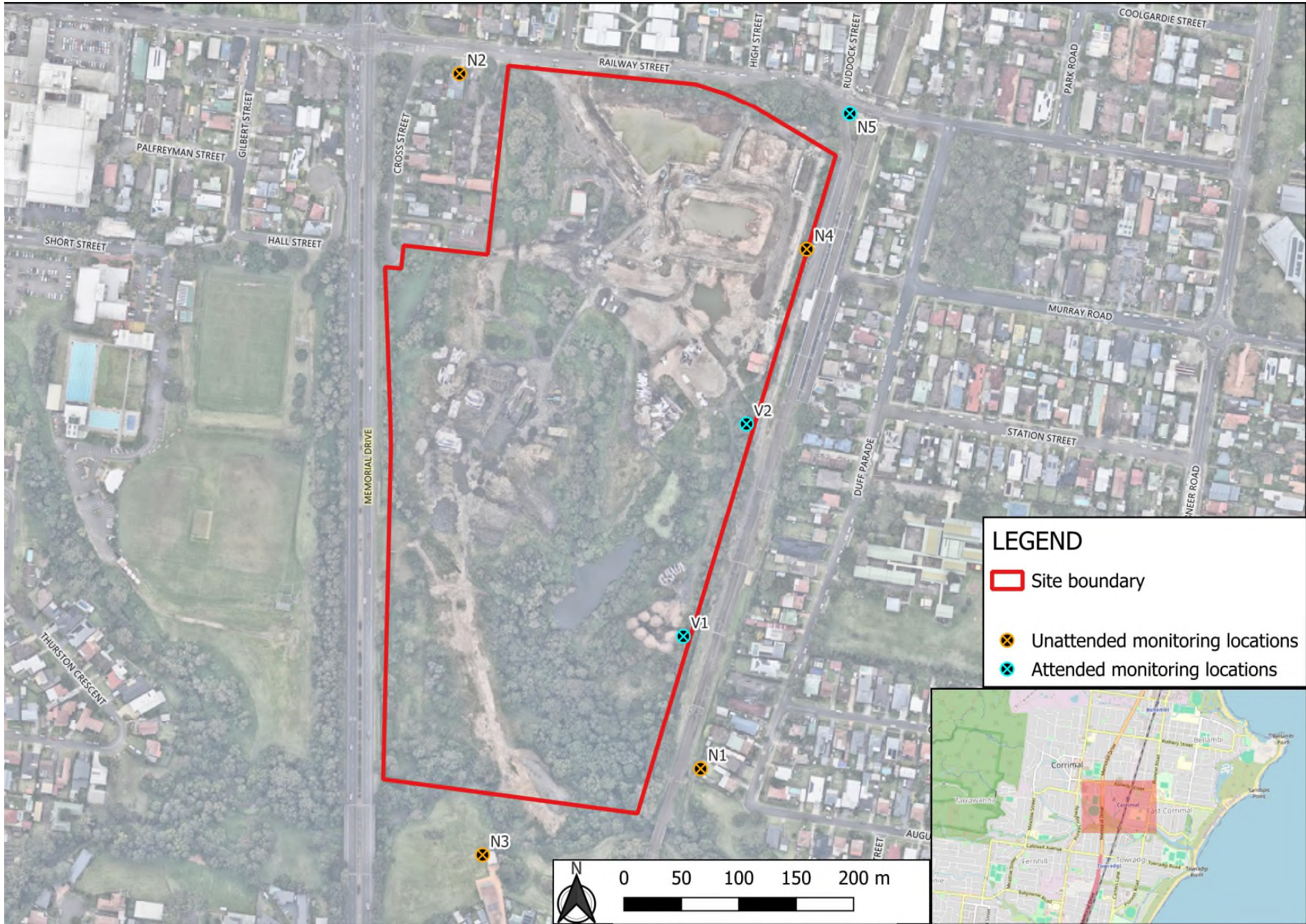
Figure 1: Noise and vibration measurement locations
