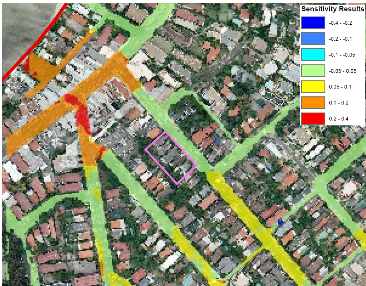
Plate 3 Impacts on peak flood level in the vicinity of the development site as a result of a 20% increase in rainfall intensity 'Rose Bay Catchment Flood Study' (WMA Water, 2010)
