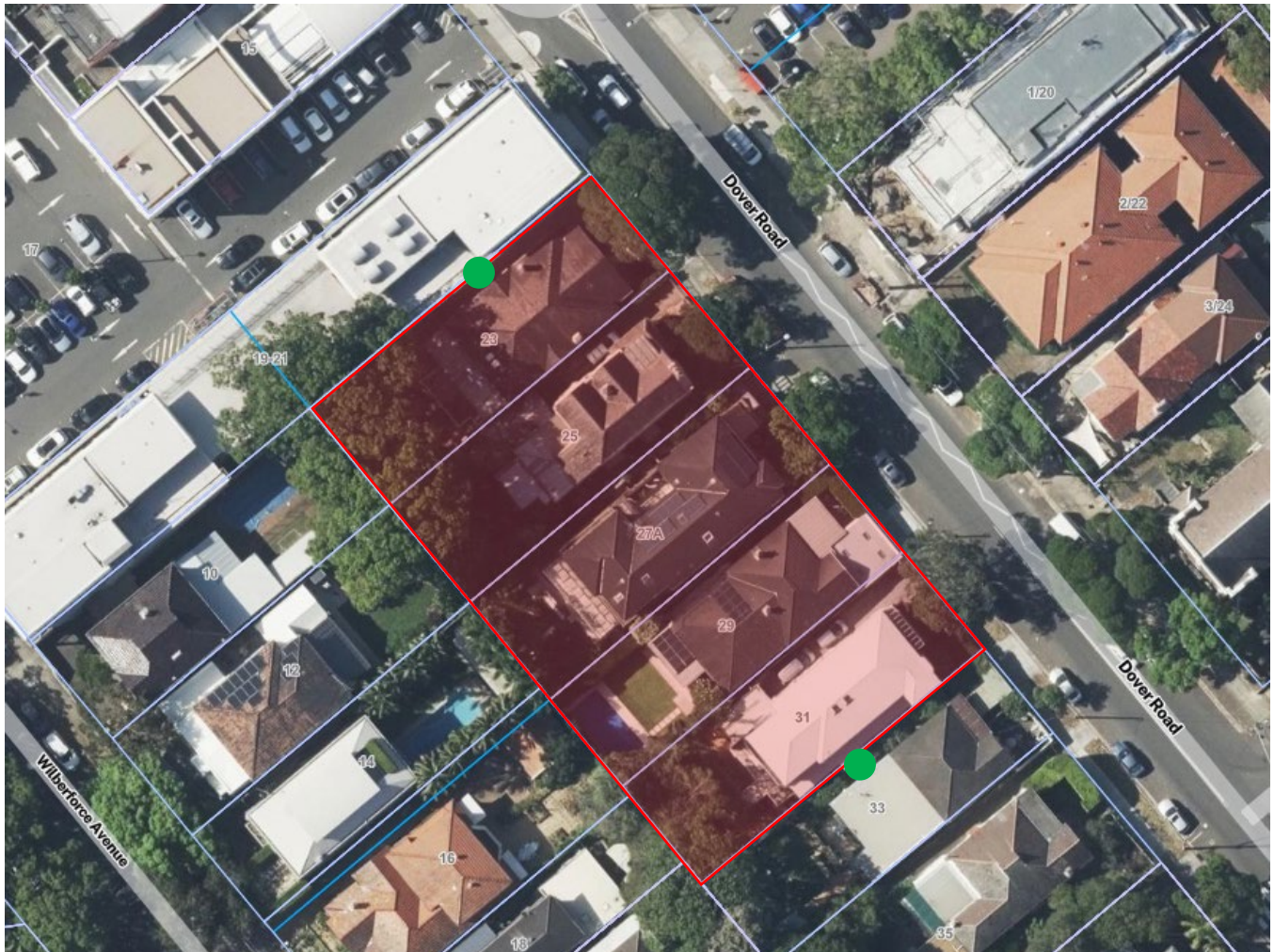
Figure 1: Location of vibration monitoring points
