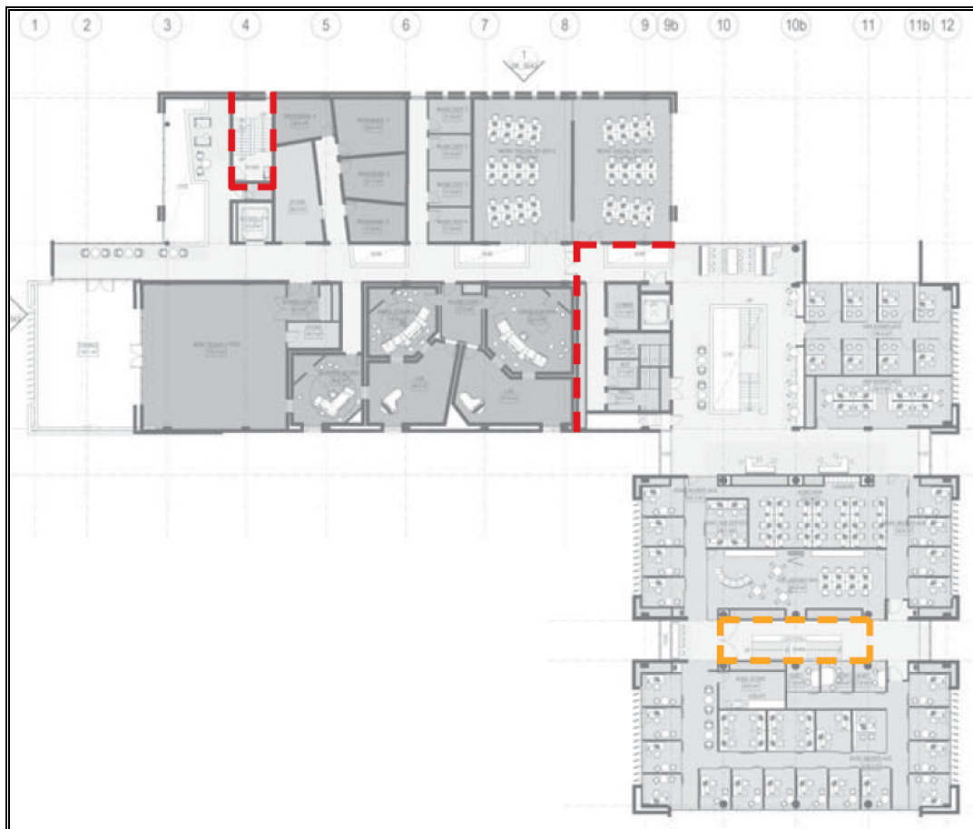
Figure 50 – Level 3 Fire Compartments.
