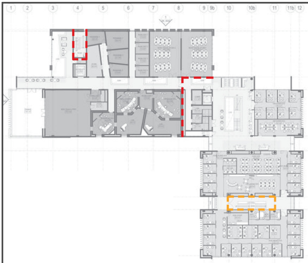
Figure 25 – Level 3 Fire Compartments.
