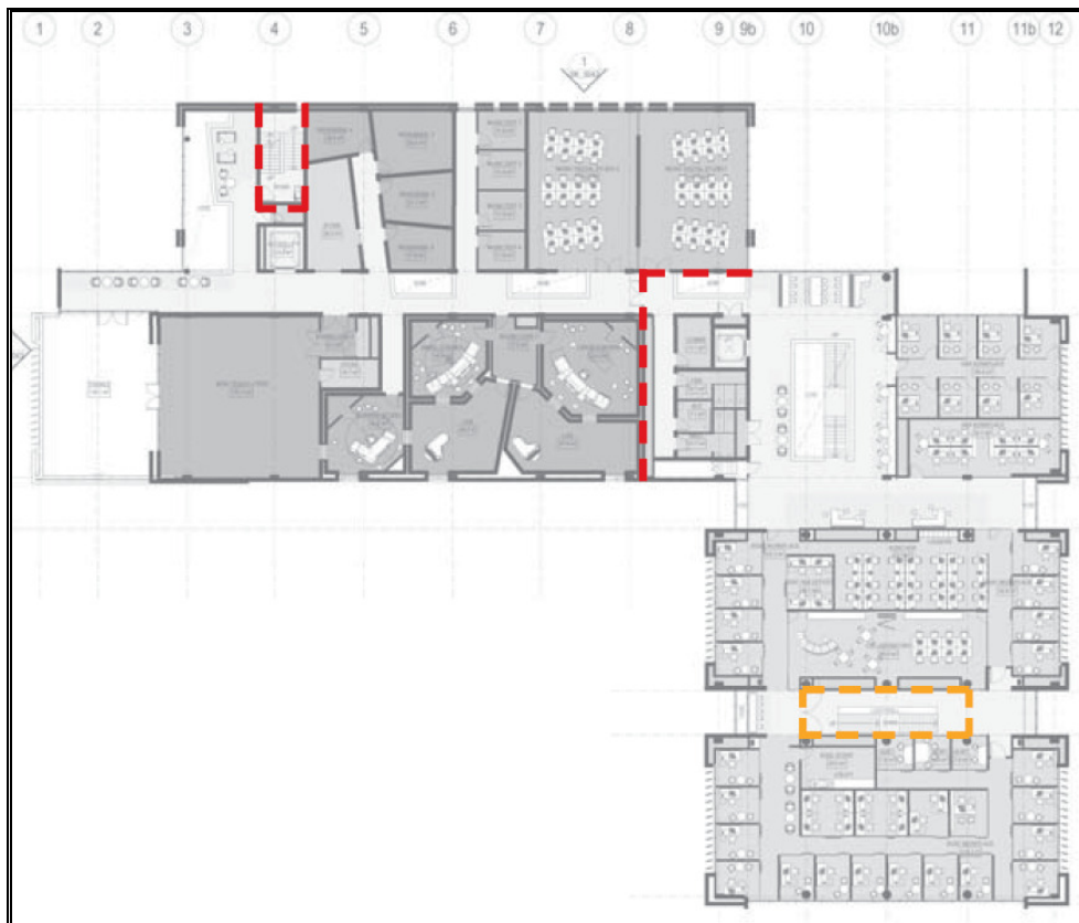
Figure 19 – Level 3 Fire Compartments.
