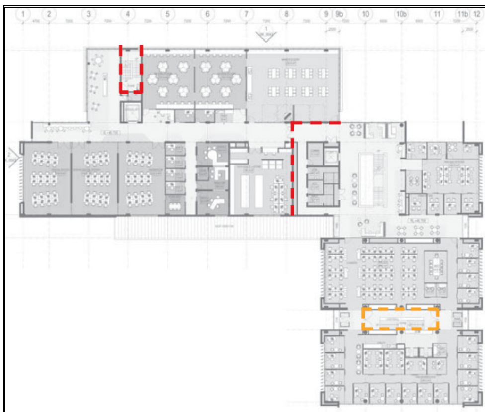
Figure 49 – Level 2 Fire Compartments.
