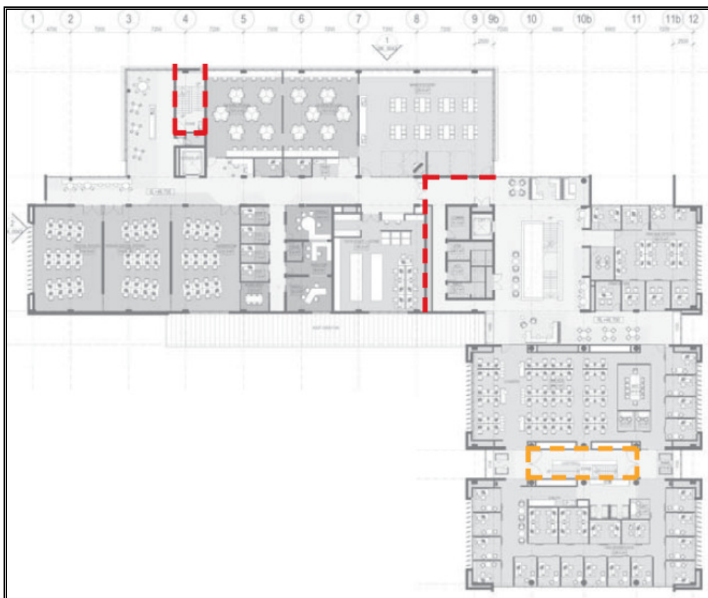
Figure 24 – Level 2 Fire Compartments.
