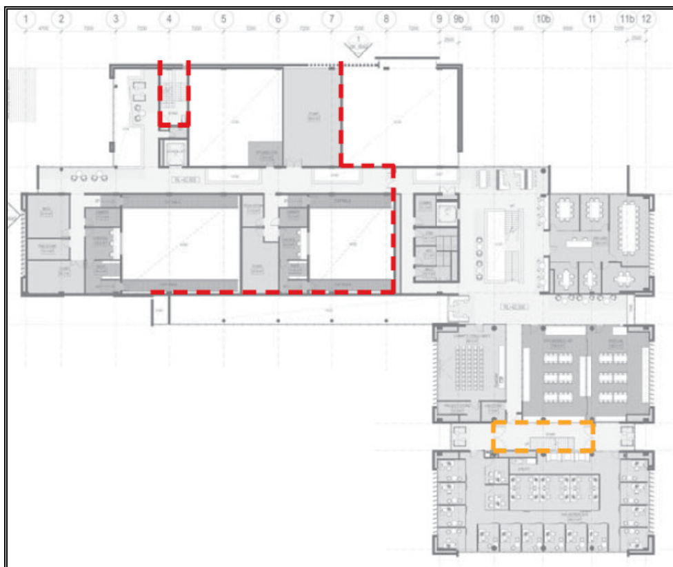
Figure 48 – Level 1 Fire Compartments.
