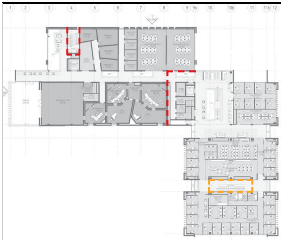
Figure 4 – Level 3 Fire Compartments.
