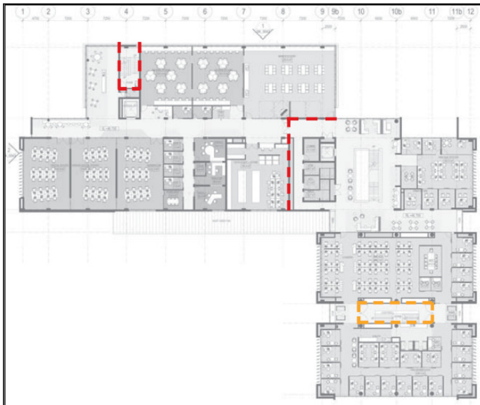
Figure 3 – Level 2 Fire Compartments.
