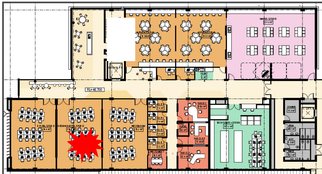
Figure 124 – Uncontrolled fire scenario inside Level 2 North fire compartment.
