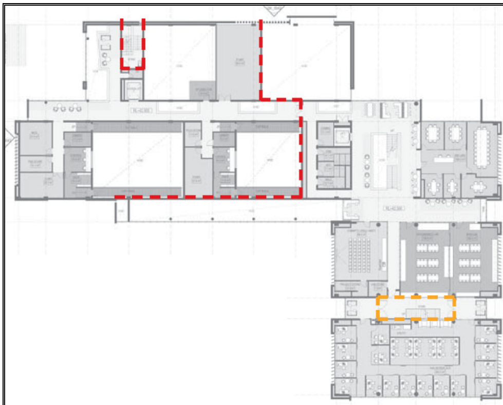
Figure 38 – North fire-isolated stairway and east fire-isolated stairway subject of this assessment.
