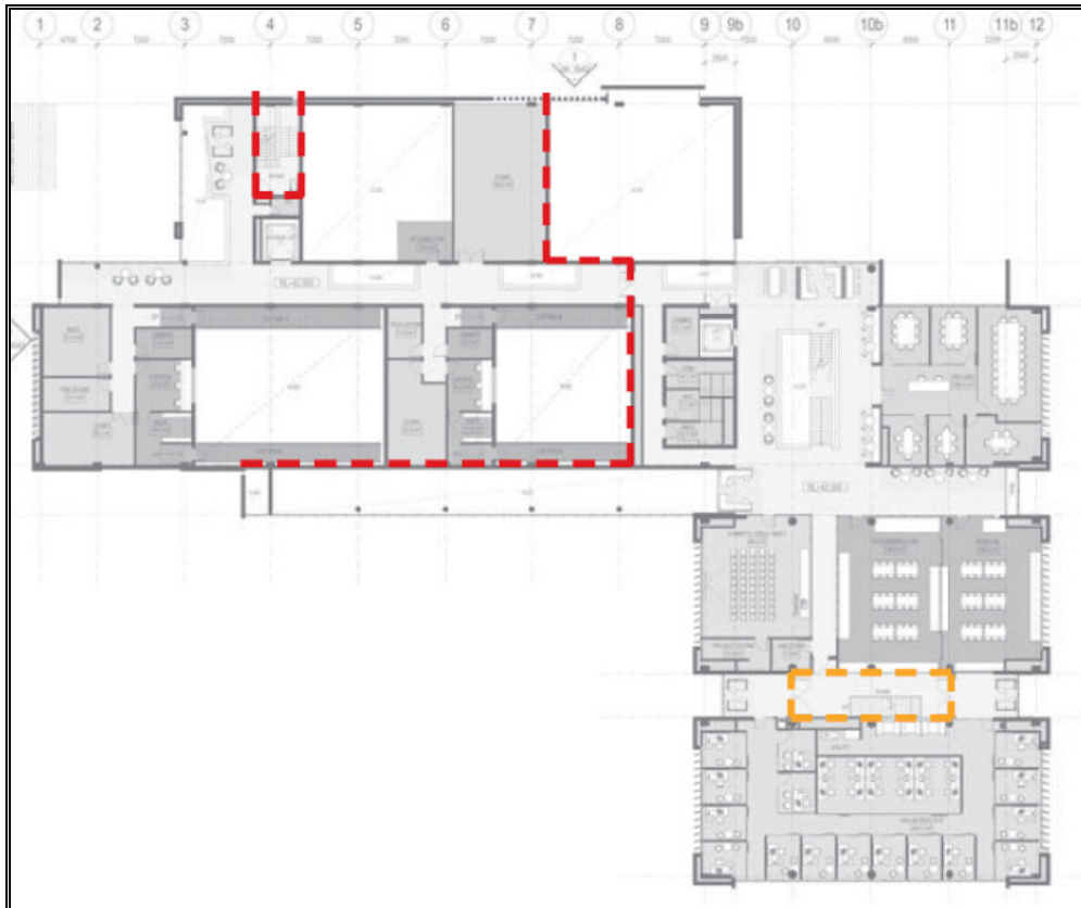
Figure 23 – Level 1 Fire Compartments.
