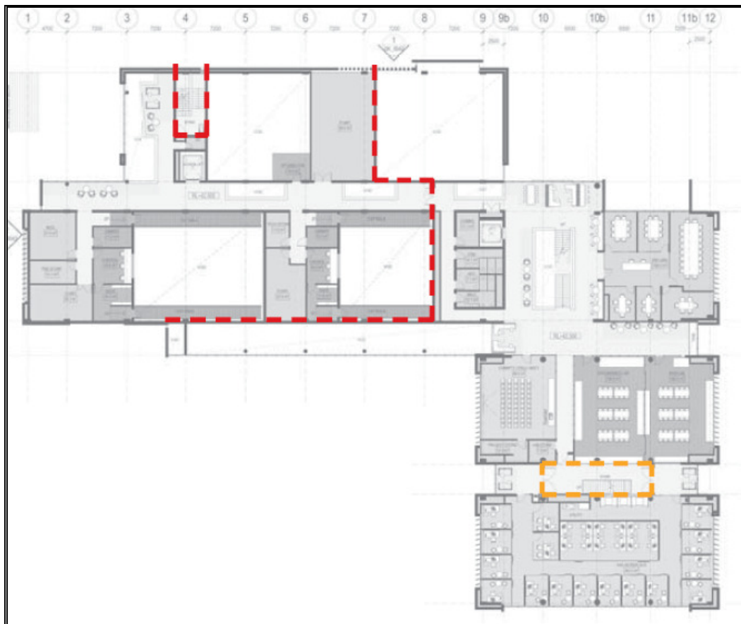
Figure 2 – Level 1 Fire Compartments.
