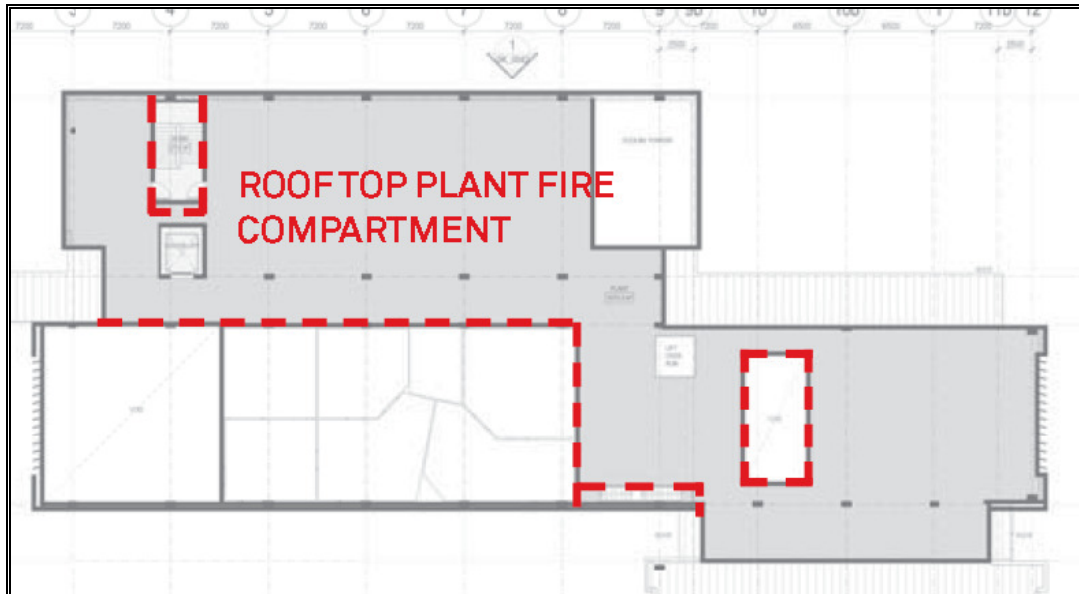
Figure 5 – Level 4 (Plants) Fire Compartments.
