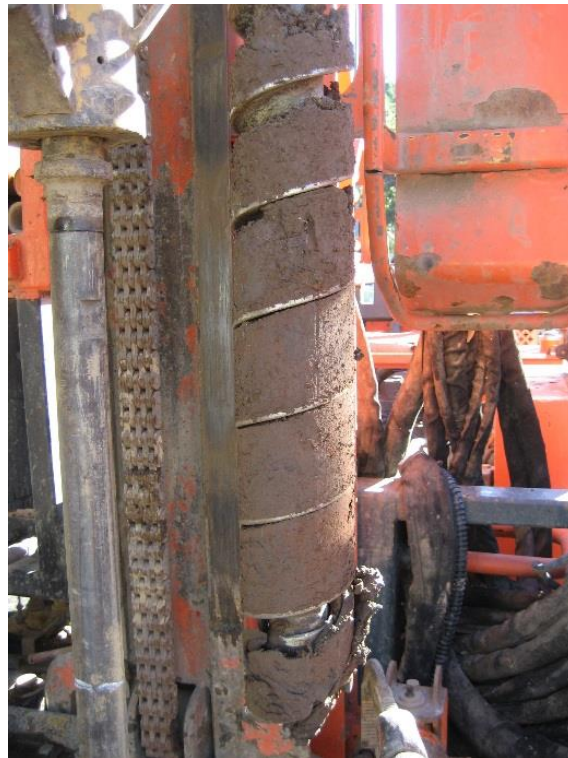
Photo 12: Typical alluvial material retrieved from CBH01 at a depth of about 2.0m to 3.0m, showing high plasticity clay.
