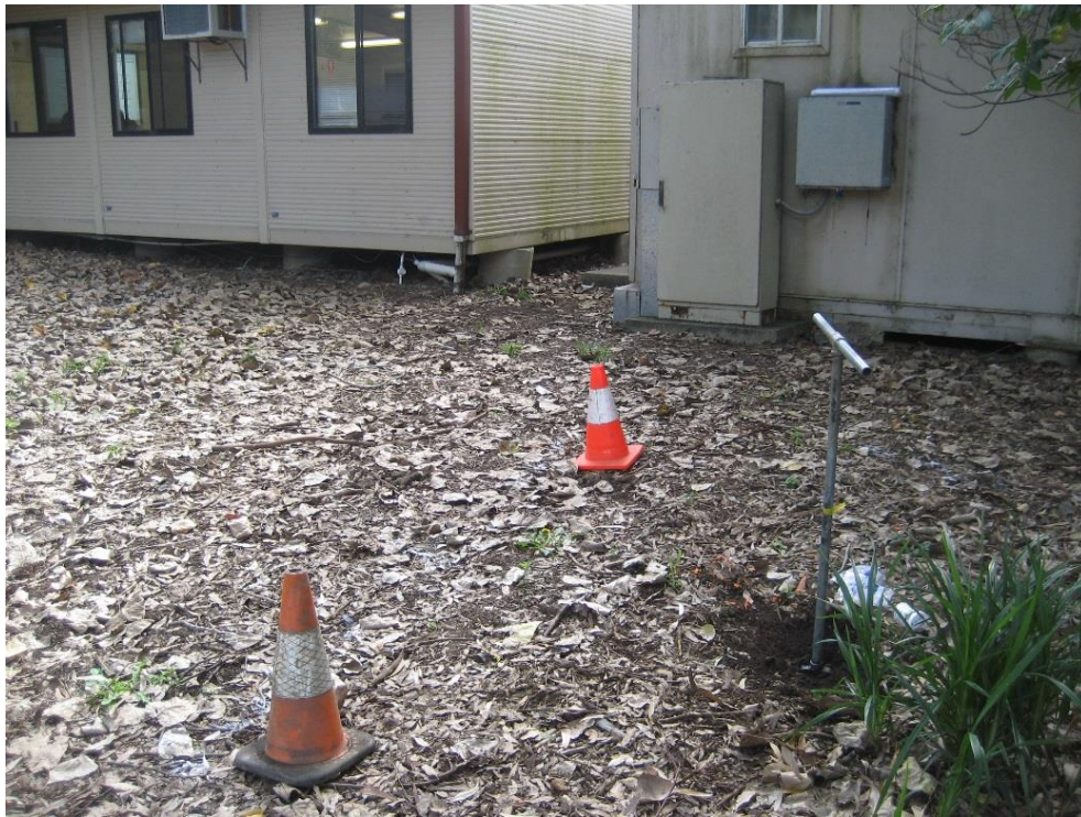
Photo 16: View of the borehole CBH05. Due to existing several underground services, borehole was drilled only to shallow depth by hand auger.
