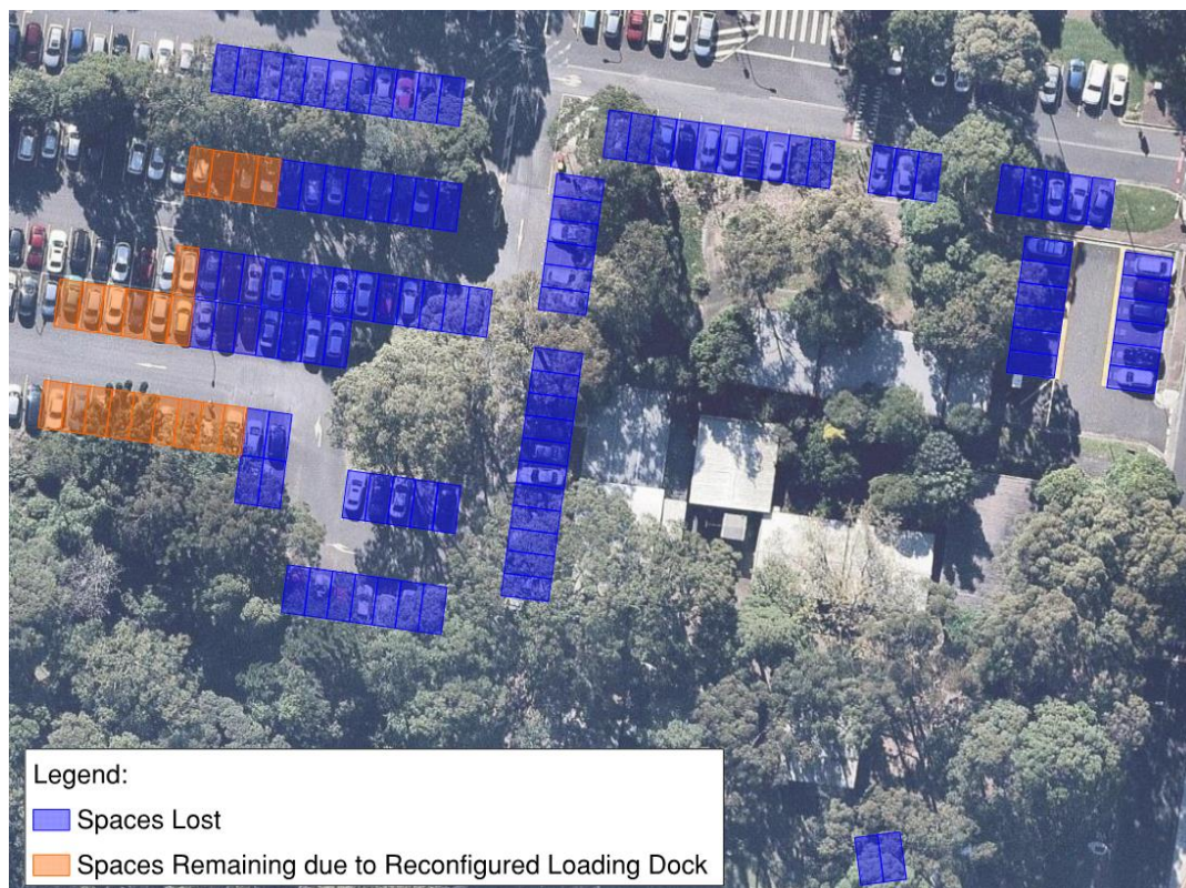
Figure 1: Parking Loss due to Reconfigured Loading Dock
