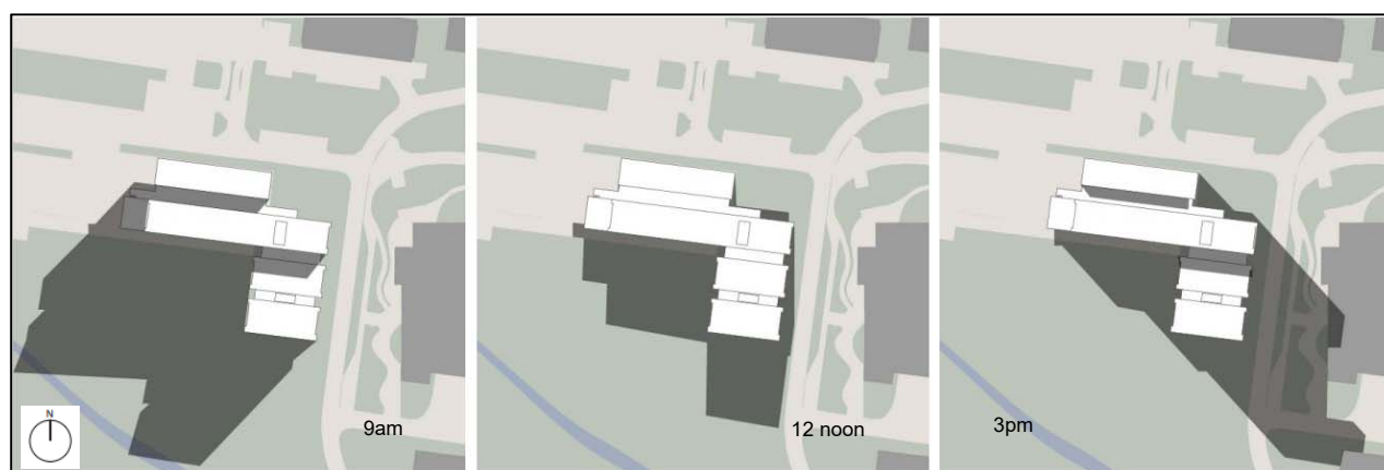
Figure 20: Shadow Diagram of the Winter solstice at 9am, 12 noon and 3pm on 21 June (source: EIS)
