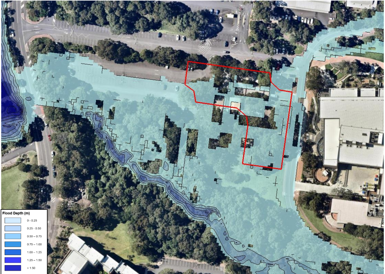
Figure 2-1 Existing 100 year ARI Flood Depth and Extent
