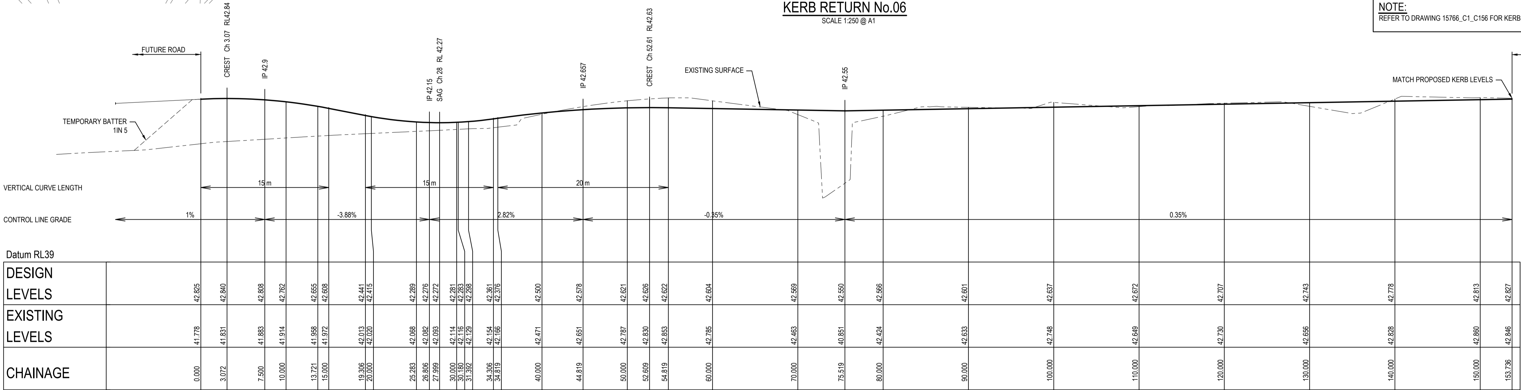
LONGITUDINAL SECTION KERB RETURN No.06 - LIP OF KERB
