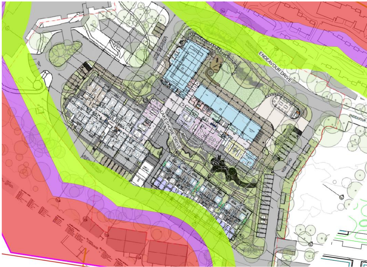
Figure 07: Proposed Stage 1 General Arrangement Plan Overlaid with BAL FZ (Red), BAL 40 (Purple) and BAL 29 (Green)
