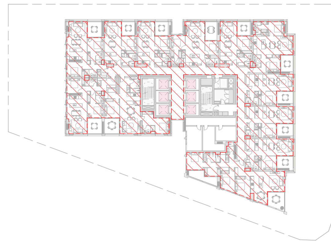
1 GFA - LEVEL 33 1 : 500 Commercial GFA: - Retail GFA: - Residential BTS GFA: 1018 m 2 Residential AH GFA: -
