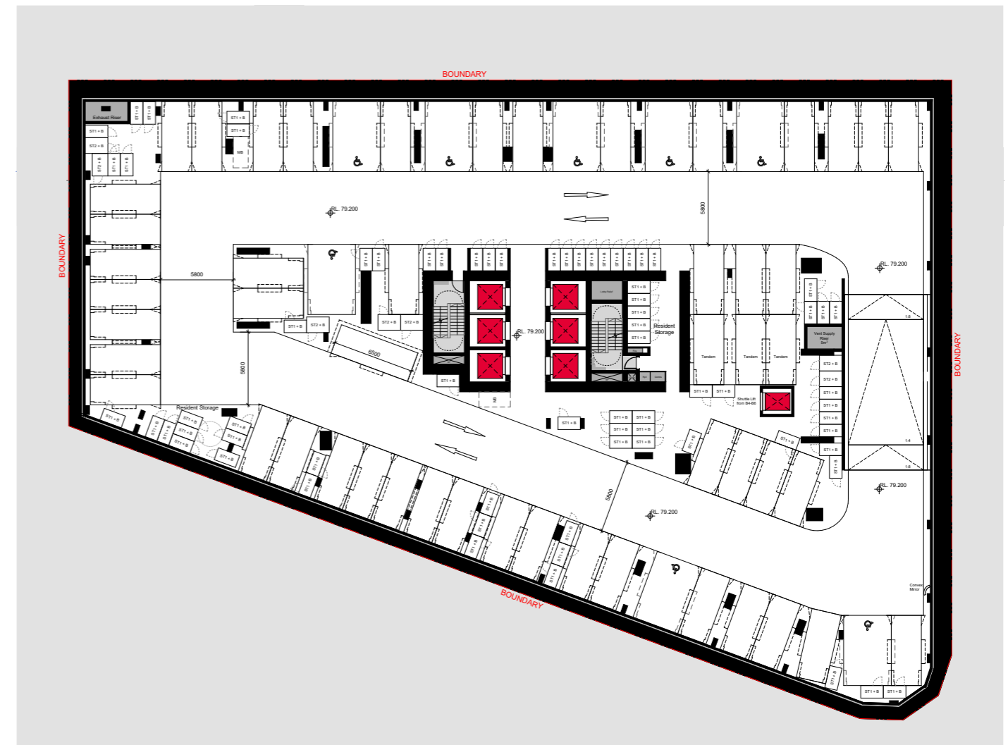
Typical Basement Level
