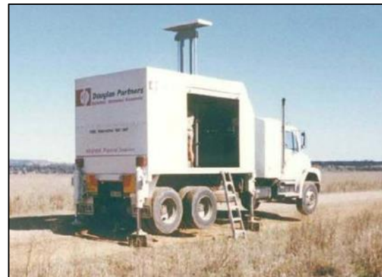
Figure 2: Purpose built CPT rig
