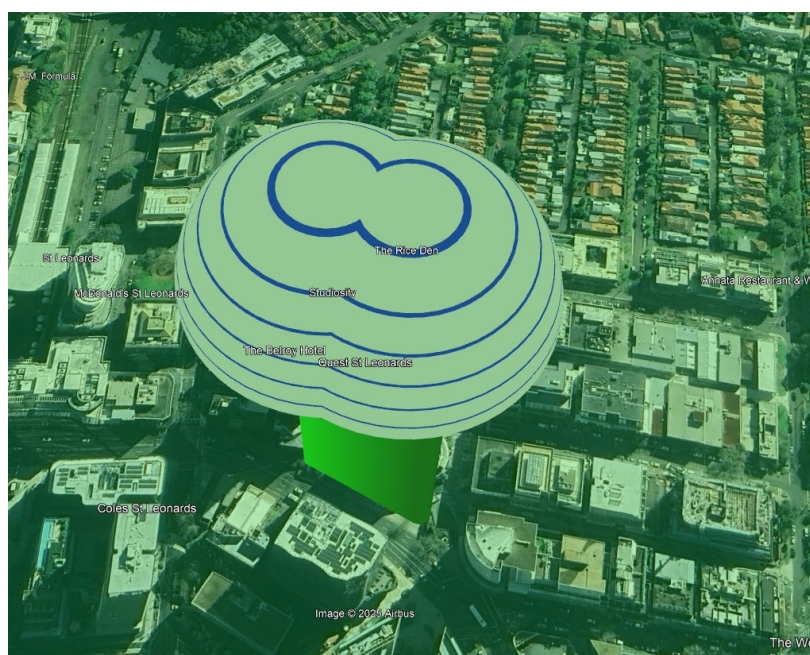
Figure 16: Avlaw's model of the proposed building and two (2) tower luffing cranes below the RTCC
