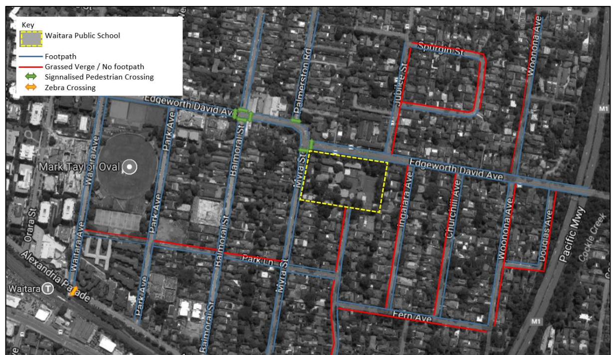
Figure 2-10 – Pedestrian Facilities in Proximity to Waitara Public School
