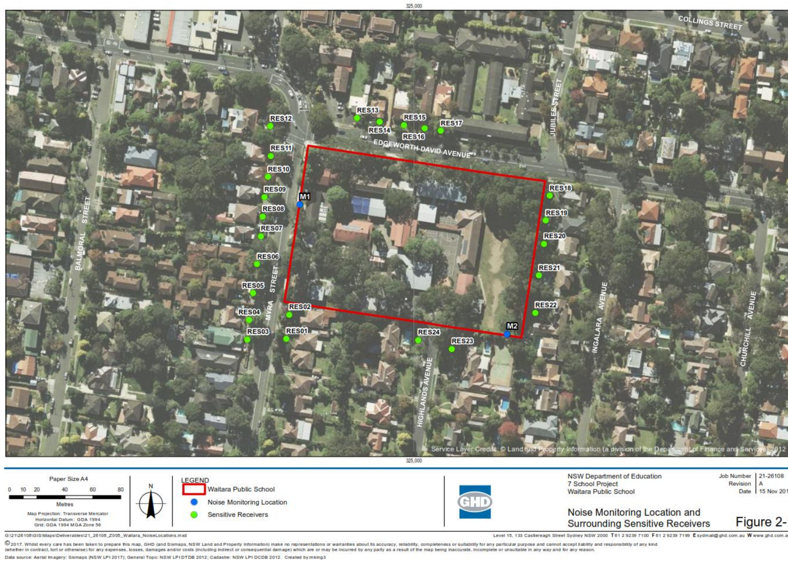
Figure 2-1 Noise monitoring location and surrounding sensitive receivers
