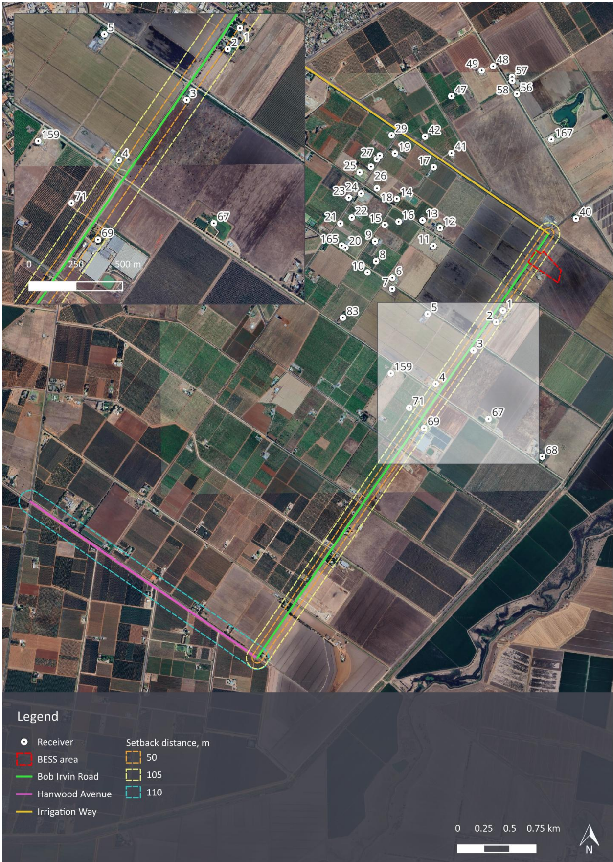
Figure 7: Receivers within minimum setback distances adjacent to assessed roads – Project & YSF & HRSFB
