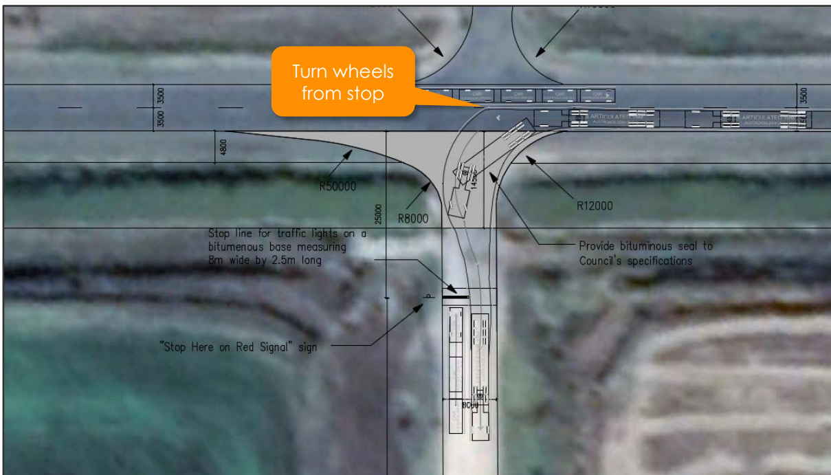
Figure 5 ML Traffic Engineers Swept Path Extract
