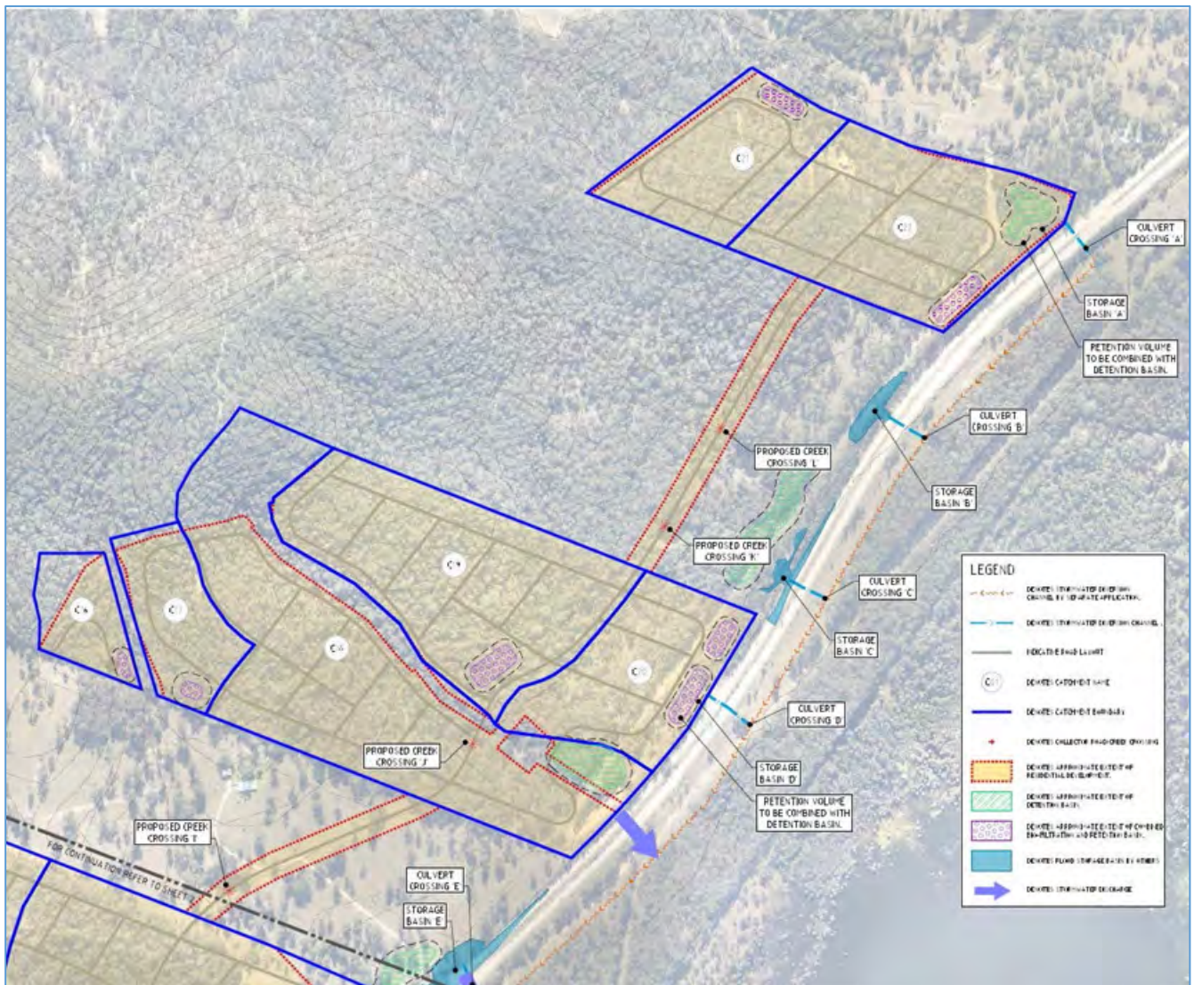
Figure 74 Proposed stormwater management – northern catchments
