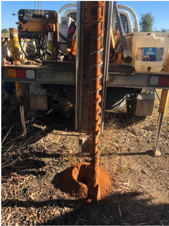
Figure 25. SP1 borehole displaying dry, natural soil
