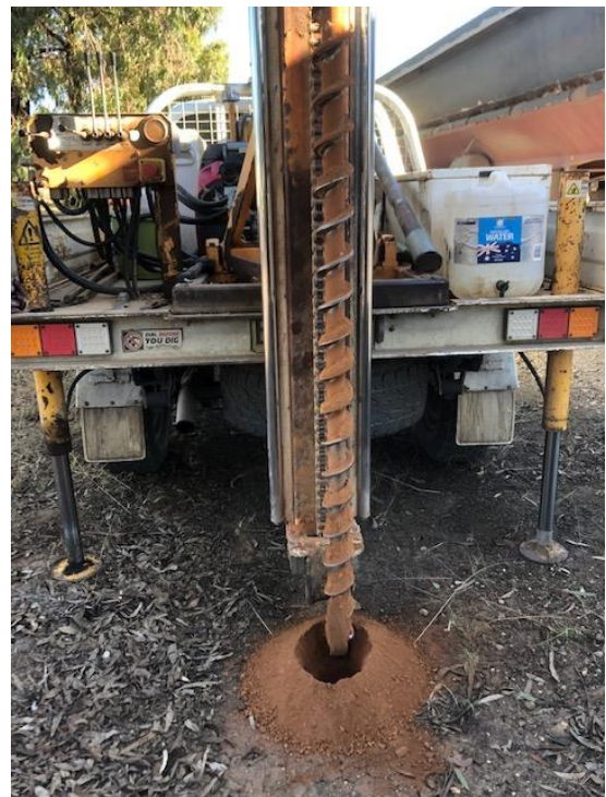
Figure 26. SP2 borehole displaying dry, natural soil
