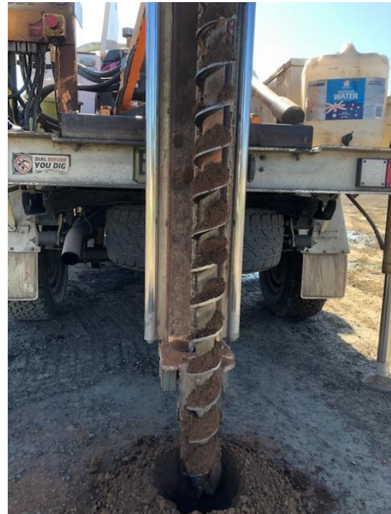
Figure 30. SP6 borehole displaying moister soil beneath 50mm of road base.
