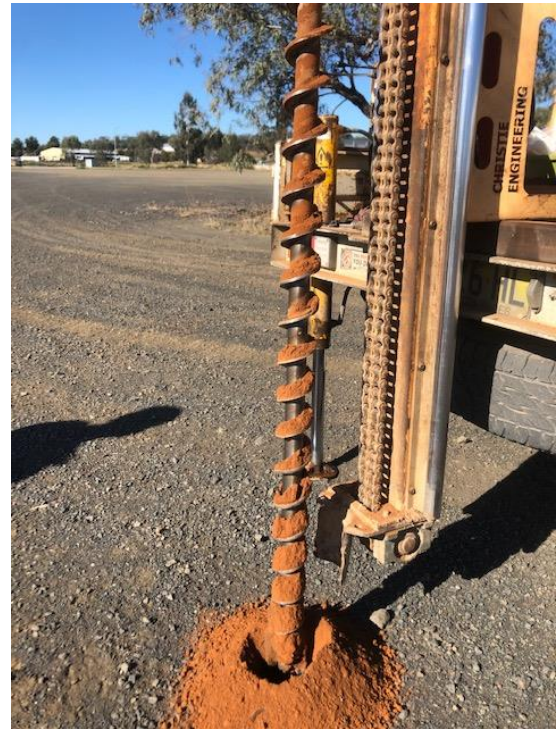
Figure 38. SP14 borehole displaying dry, natural soil beneath 50mm of road base
