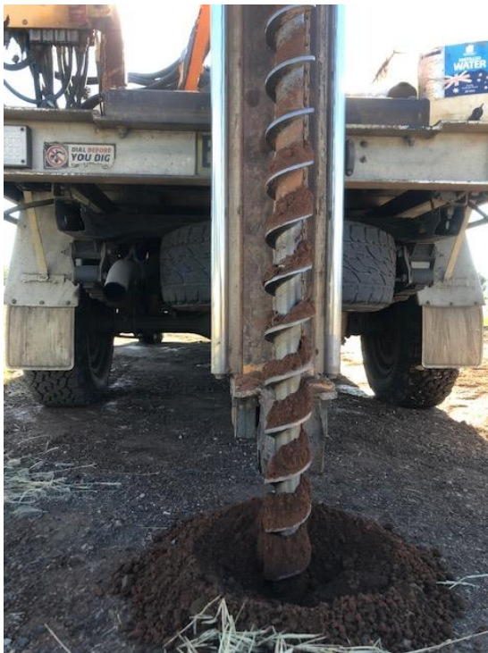
Figure 31. SP7 borehole displaying moist, natural soil beneath 50mm of road base
