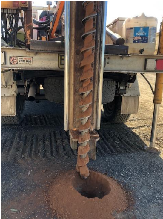
Figure 29. SP5 borehole displaying dry, natural soil beneath 50mm of road base
