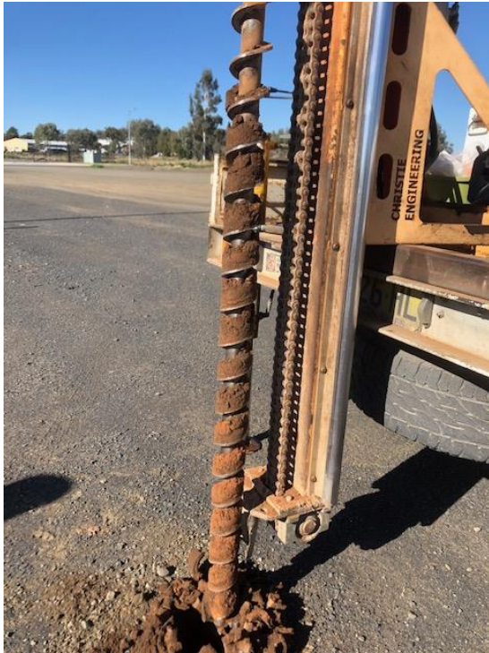
Figure 37. SP13 borehole displaying moist, natural soil beneath 10mm of road base
