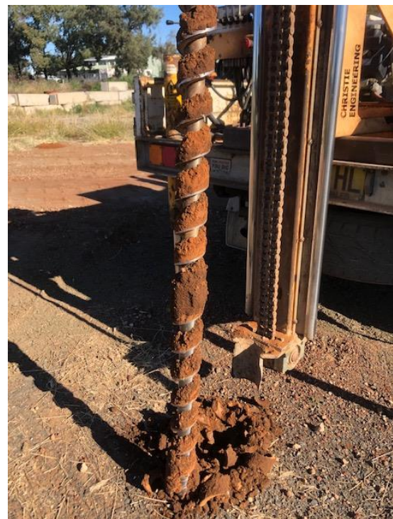
Figure 32. SP8 borehole displaying moist, natural soil beneath 50mm of road base
