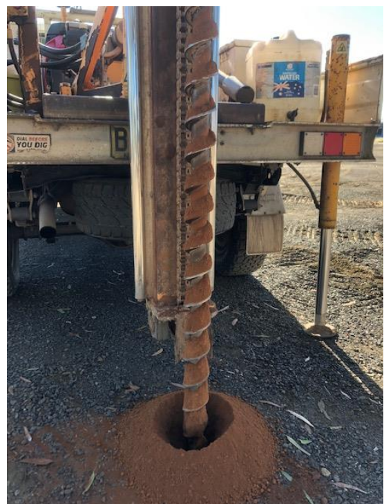
Figure 28. SP4 borehole displaying dry, natural soil beneath 50mm of road base
