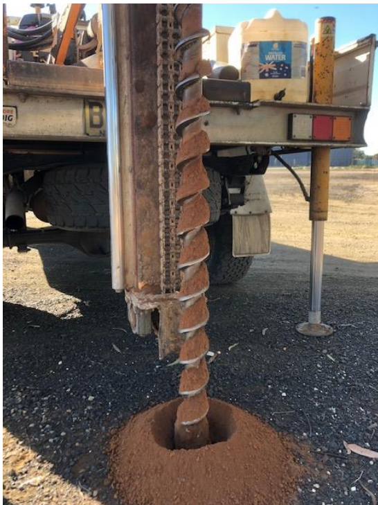
Figure 27. SP3 borehole displaying dry, natural soil beneath 50mm of road base
