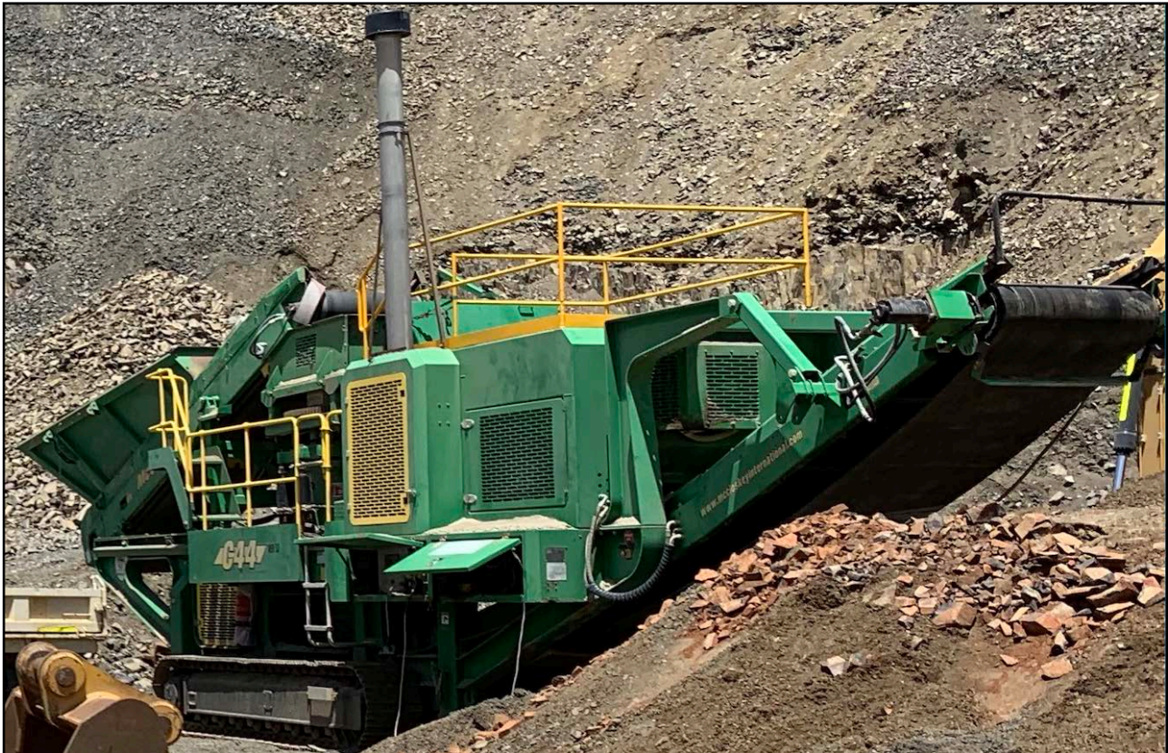
PHOTOGRAPH 3.6 (above): Typical crushing plant at MEX Marys Mount Quarry (McCloskey J50 shown in photo), to be used on a campaign basis at the proposed waste facility.
