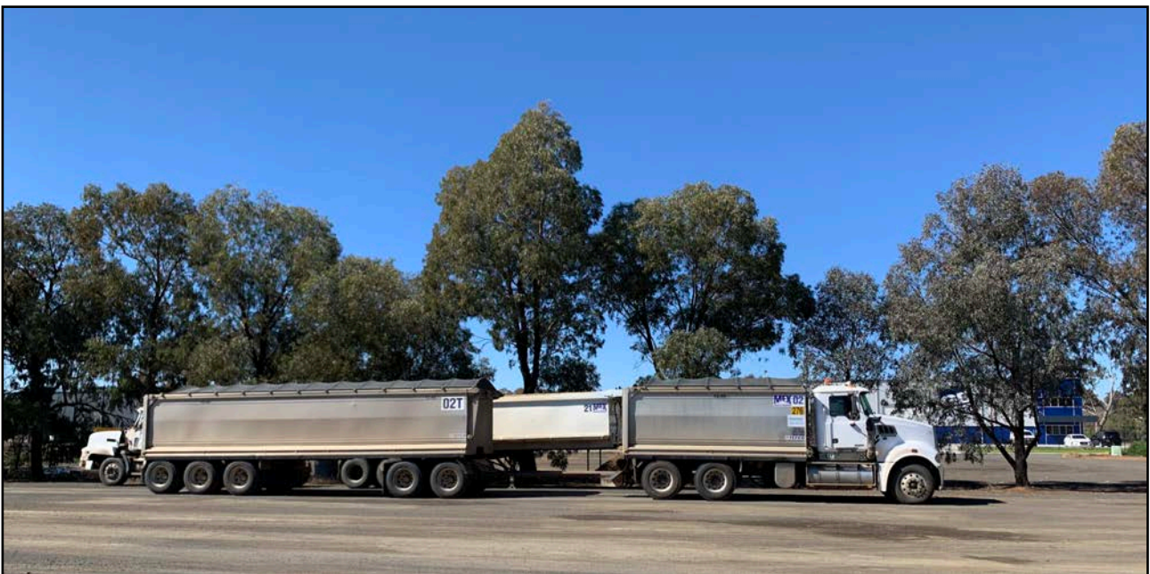
PHOTOGRAPH 3.4 (above): Typical heavy haulage vehicle- 8 axle truck and dog articulated heavy vehicle with a current lawful payload of up to 45 tonnes. View of MEX trucks in existing hardstand truck parking area on the project site, with existing landscaping and GB Autos building in rear.
