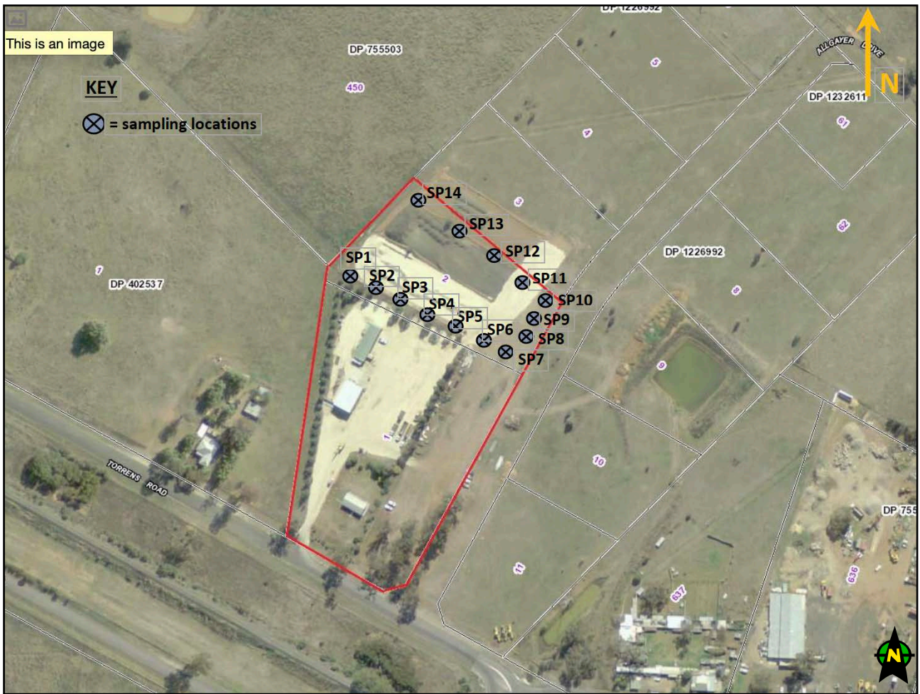
FIGURE 4.25: Extent of sampling locations as part of the contamination assessment
