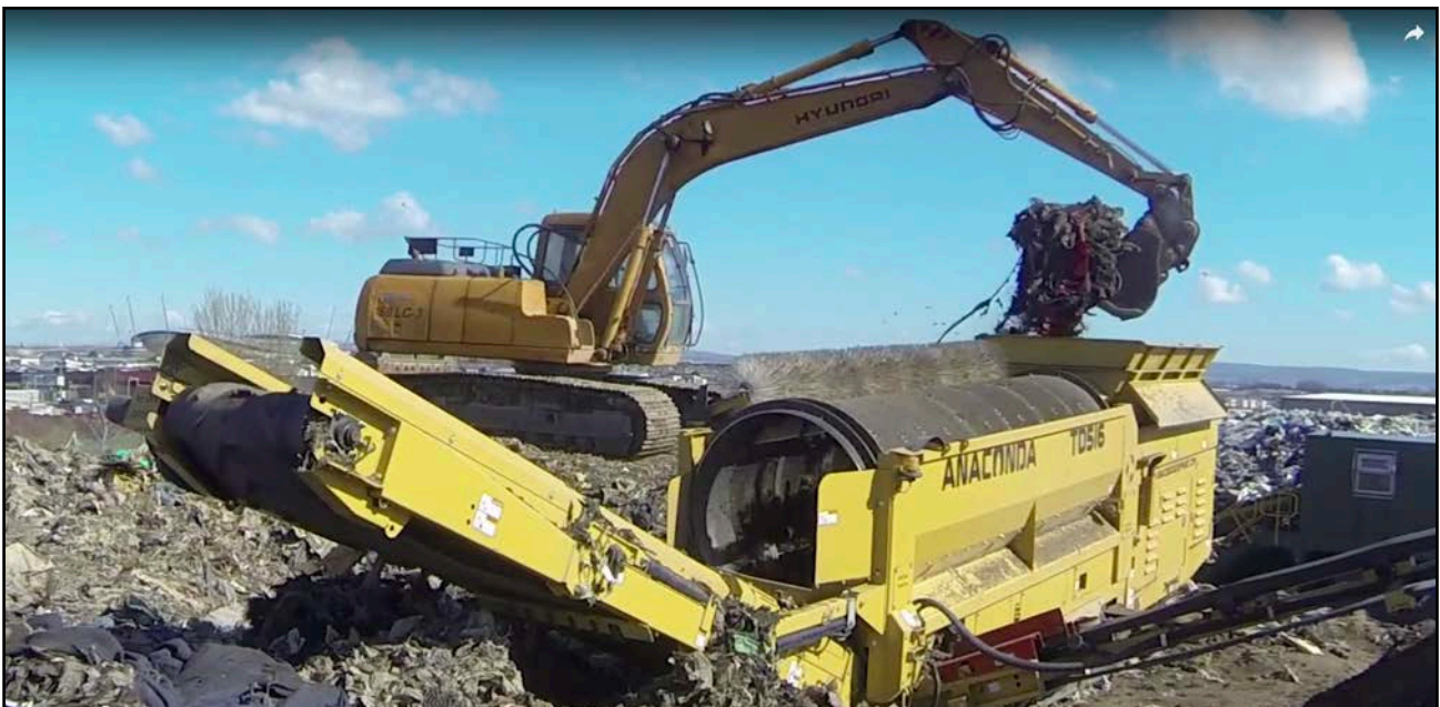
PHOTOGRAPH 3.5 (above): Loading of waste into a typical tracked trommel (Anaconda). The trommel itself is on crawler tracks and can be easily moved if required. To the left and right of the trommel are the conveyors, which deposit processed waste into stockpiles.
