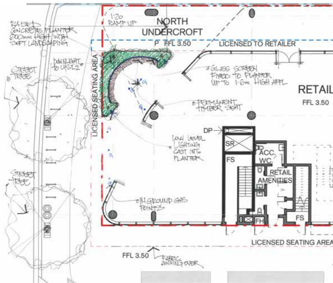
Indicative Design for Northern Seating Area with Wind Amelioration Elements Shown
