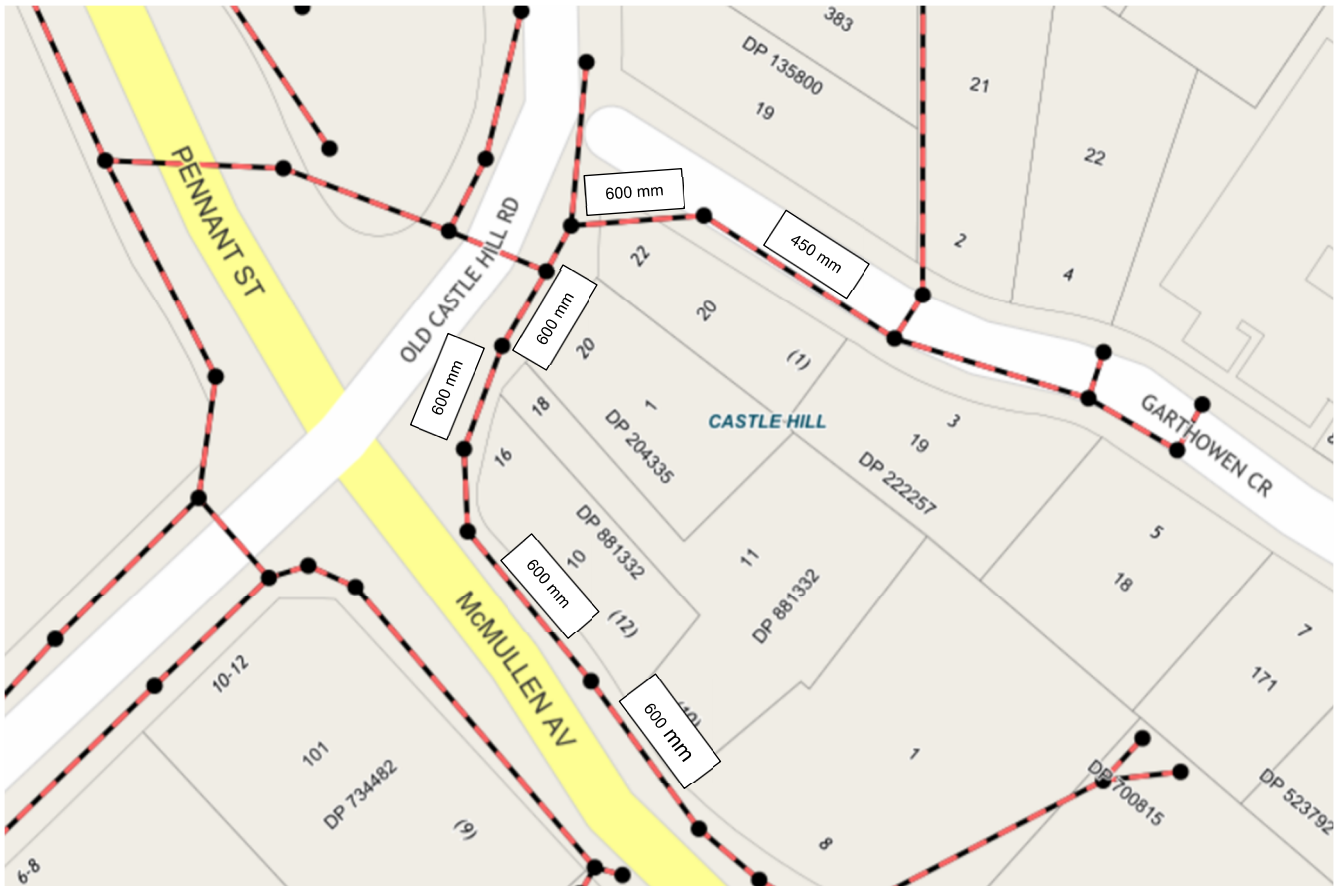
Figure 2: Existing stormwater network (GIS)
