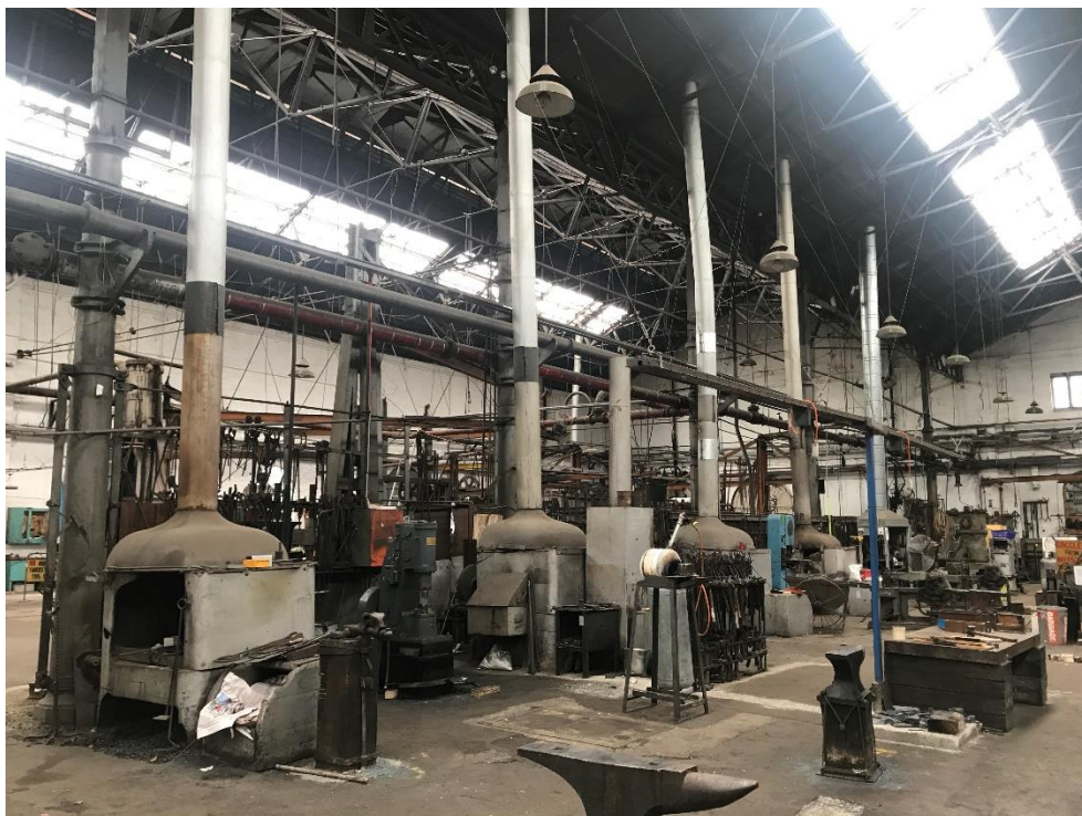
Figure 6: Furnaces in Blacksmith Tenancy in 2017, Bay 2 South Source: Curio 2017
