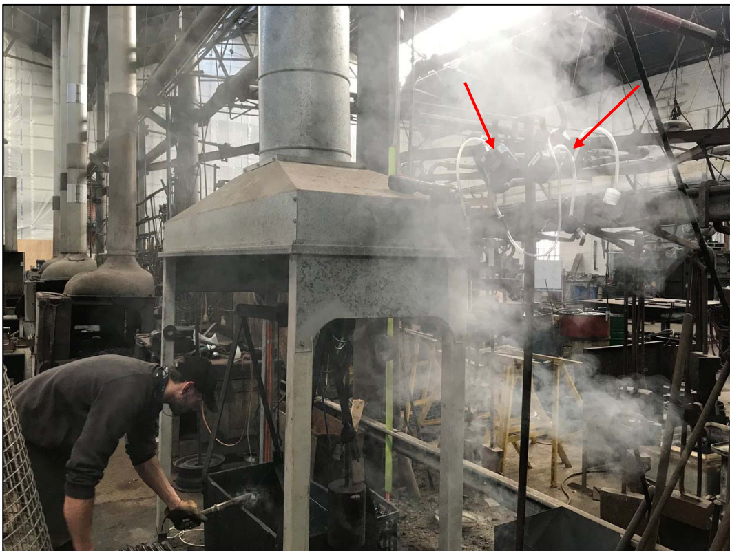
Photograph 10: Air monitoring equipment positioned in worst case exposure location during oil quenching.
