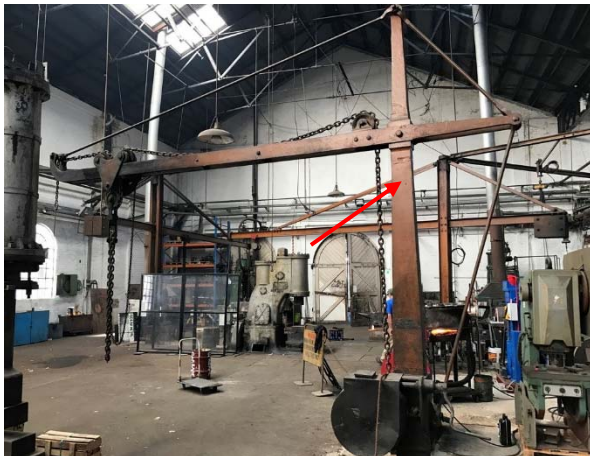
Photo 34: Bay 1 south - The orange 7 CWT Jib Crane contains lead based paint
