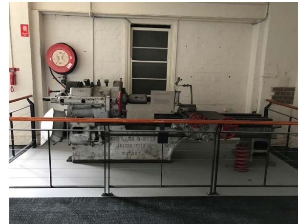
Photo 60: Bay 5 - XRF screening of the silver Johnston Spring Coiler identified lead based paint
