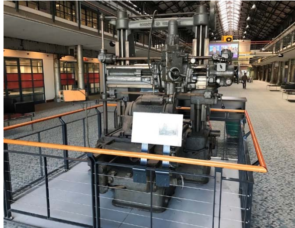
Photo 74: Bay 8 - XRF screening of the green Genevoise Drilling and Boring machines (1925 & 1938) identified lead based paints
