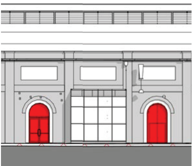
Detail - Modern large format opening, east elevation
