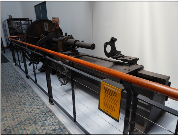
FIGURE 96: WHITLAM SPRING COILER AND SPRING SHOP RACK AND COILS IN REAR OF PHOTO, BAY 3 CENTRAL ACCESS CORRIDOR (SOURCE: CURIO 2016)
