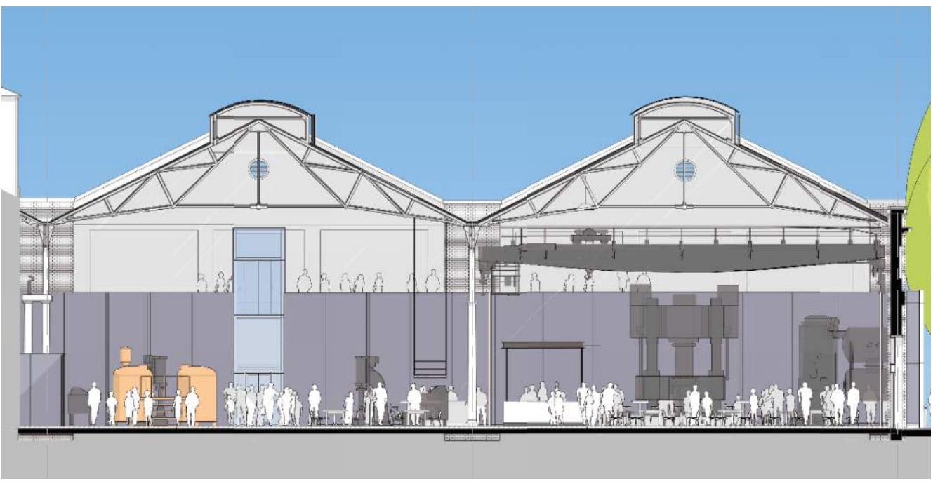
Elevation - stair and loading dock configuration Opt 2
