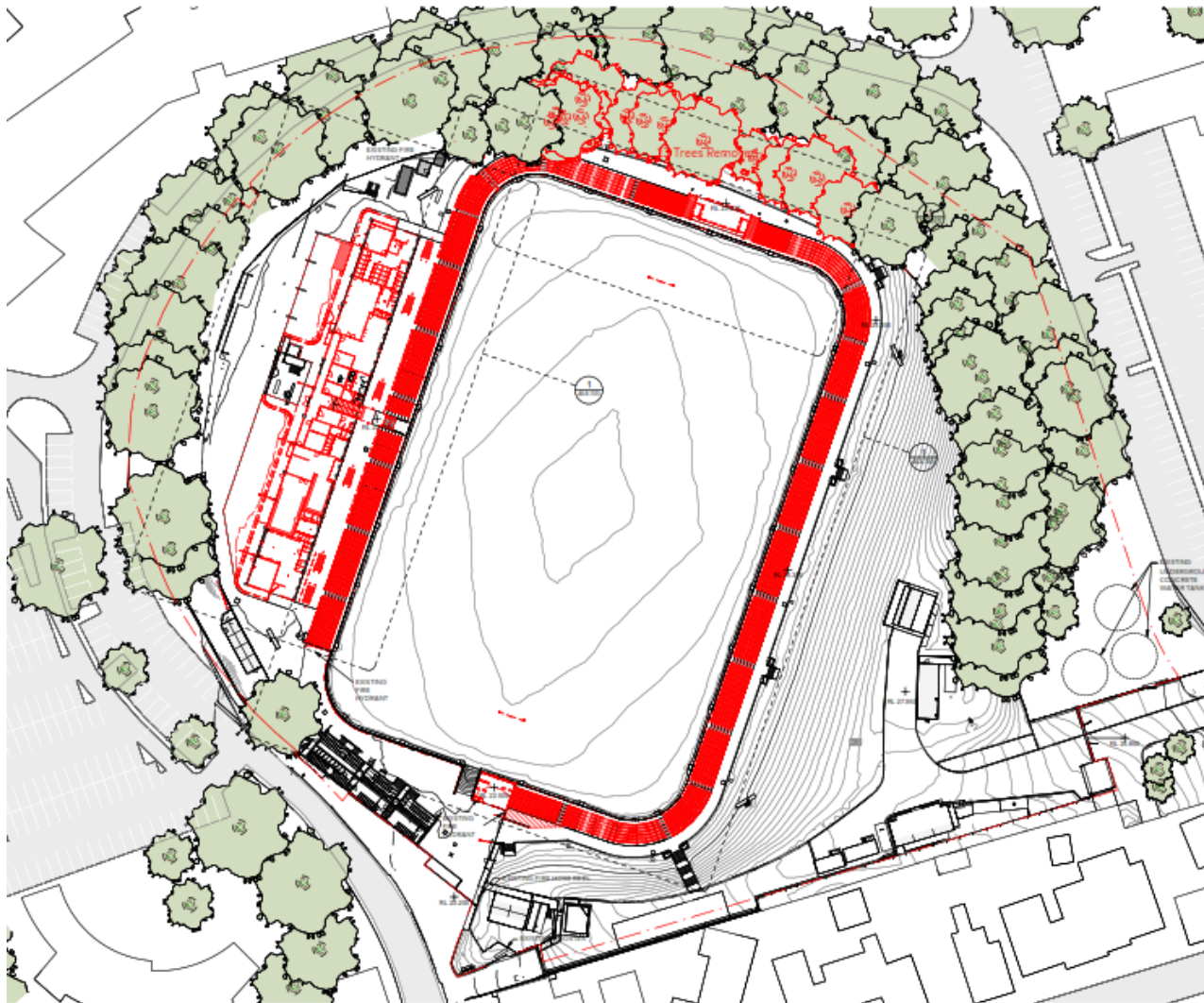
Figure 54: Proposed site demolition plan (Source: COX Architecture, 2025)
