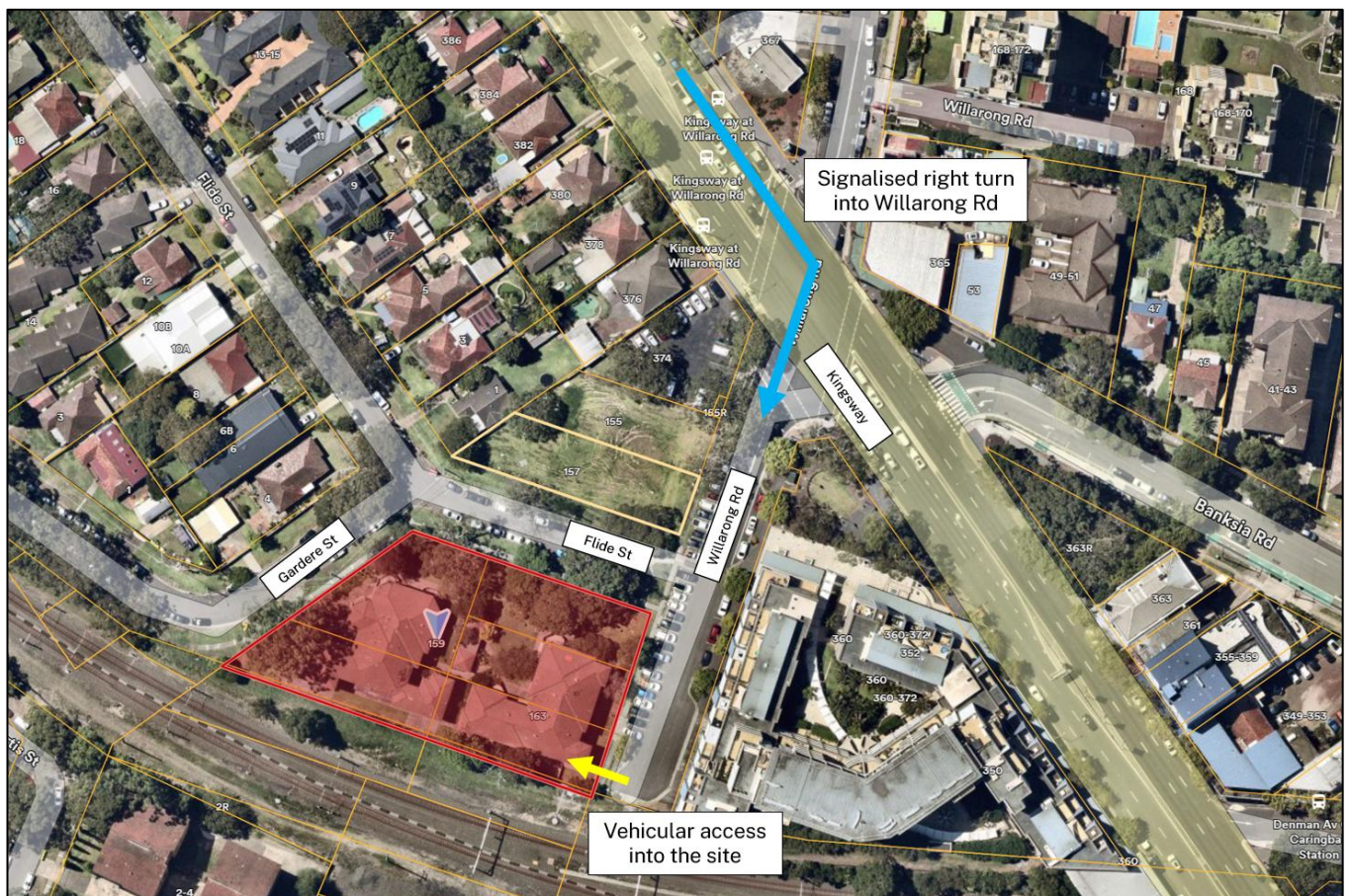
Figure 7 | Revised vehicular access route to the site, via signalised intersection from Kingsway onto Willarong Road (source: Near Map).
