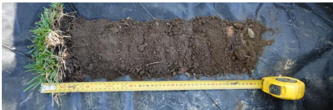
Figure 2.7 – Topsoil sample / profile, noting the refusal of the auger at 500mm depth due to the presence of rock fragments, which appear to be imported basaltic aggregates or rubble, rather than natural rock. Given this, it is anticipated that the natural soil conditions have been highly disturbed, with much of the site area excavated, and the natural soils removed (Photo: Arterra 20 March 2025)
