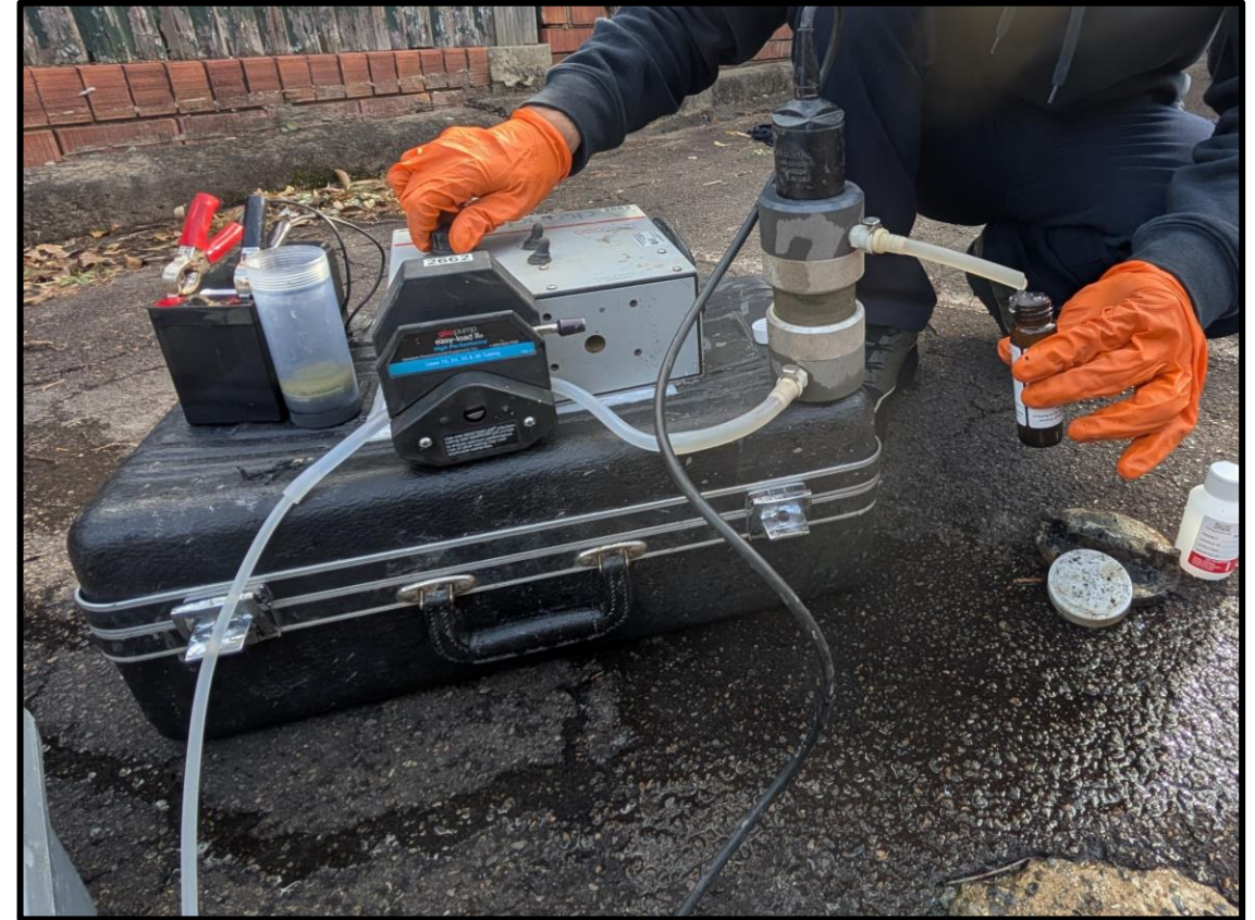
Figure 19. Micro-purging and sampling of MW2.
