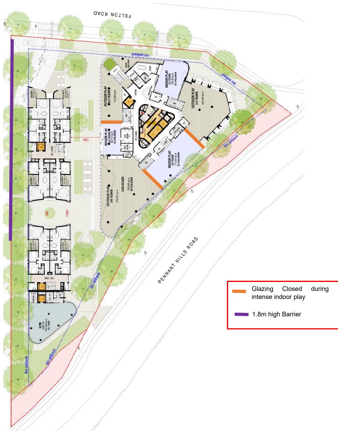
Figure 6-2 Layout of Noise Control Requirements
