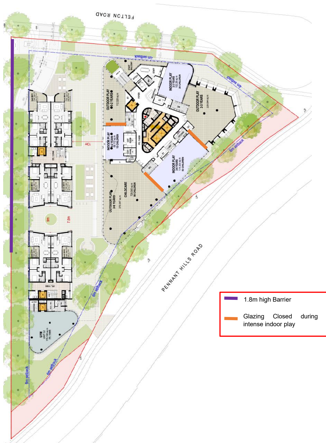
Figure 10-1 Layout of Noise Control Requirements
