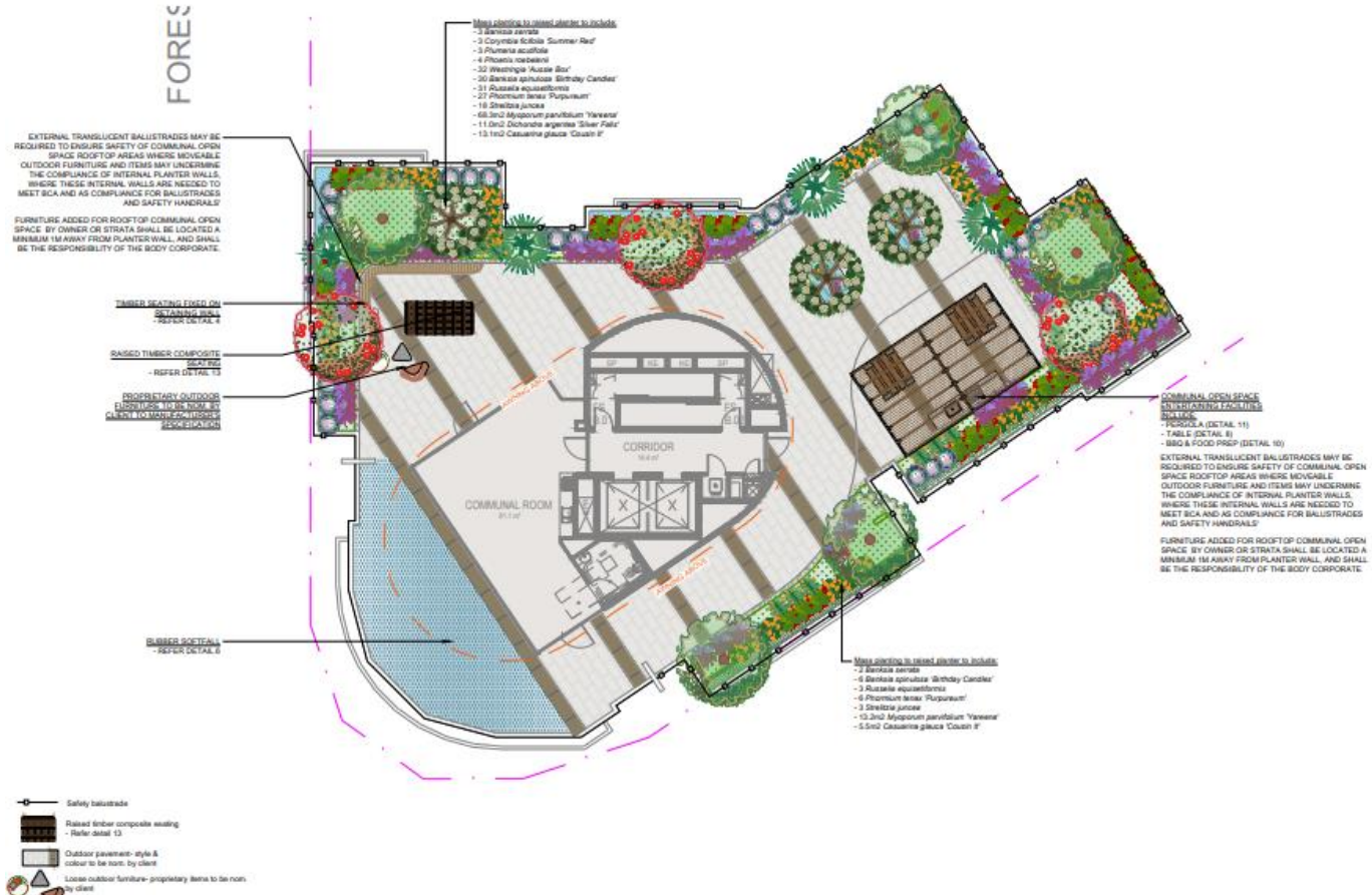
Figure 24. Roof terrace landscape plan showing the barbecue area, timber composite seating and raised planters around the perimeter (Source: Conzept Landscape Architects, 2025)
