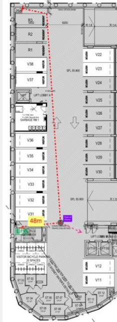
b) Extended travel distance of up to 48m in lieu of 40m to an exit.
