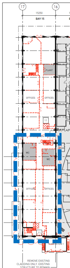
Figure 6.6: Proposed Fabric Removal Plan - Ground Floor (Source: Sissons, 2020)
