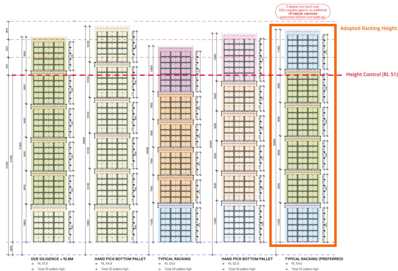
Figure 10 Typical Warehouse Racking Comparison (6-storeys)
