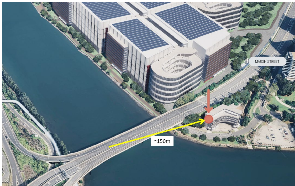
Figure 37 Driver sight distance to advertising sign
