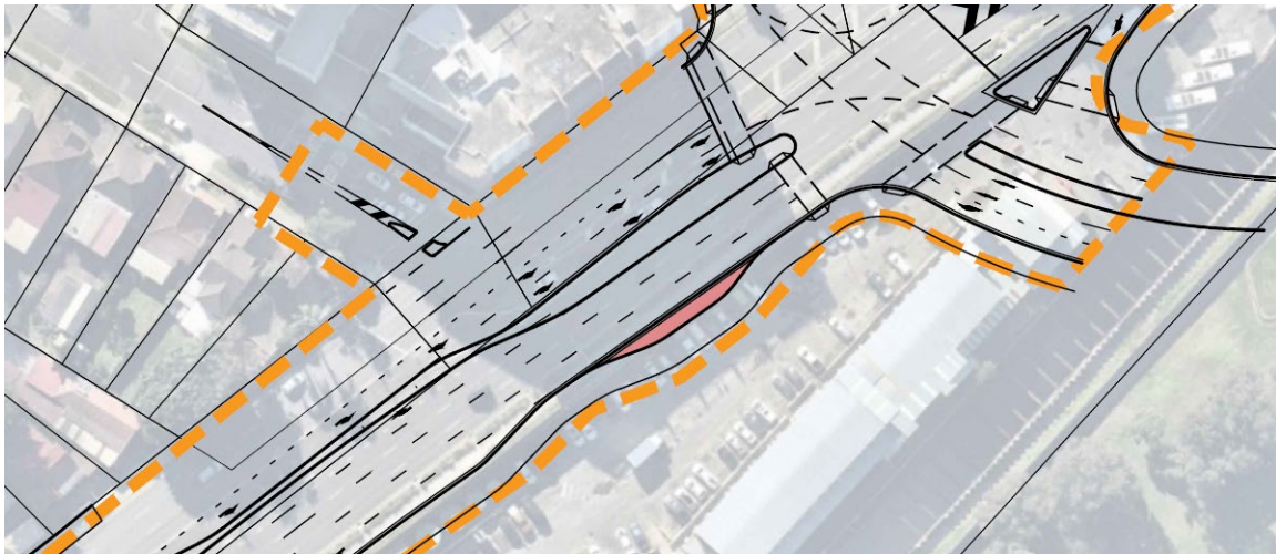
Figure 28 Southbound recessed bus bay
