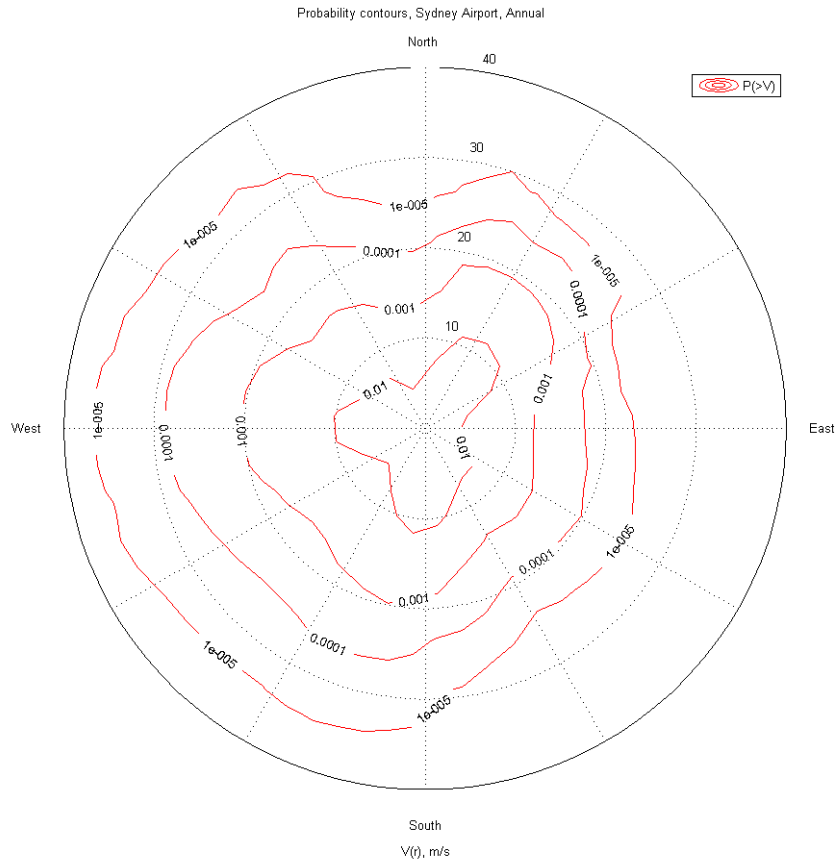
Figure 4: Wind probability of mean wind speed and direction for Sydney wind climate.
