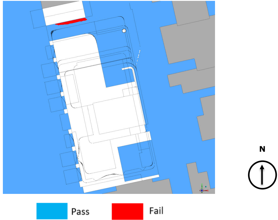
Figure 18: Wind safety result (combined all wind directions) - footpath areas and around the project site.
