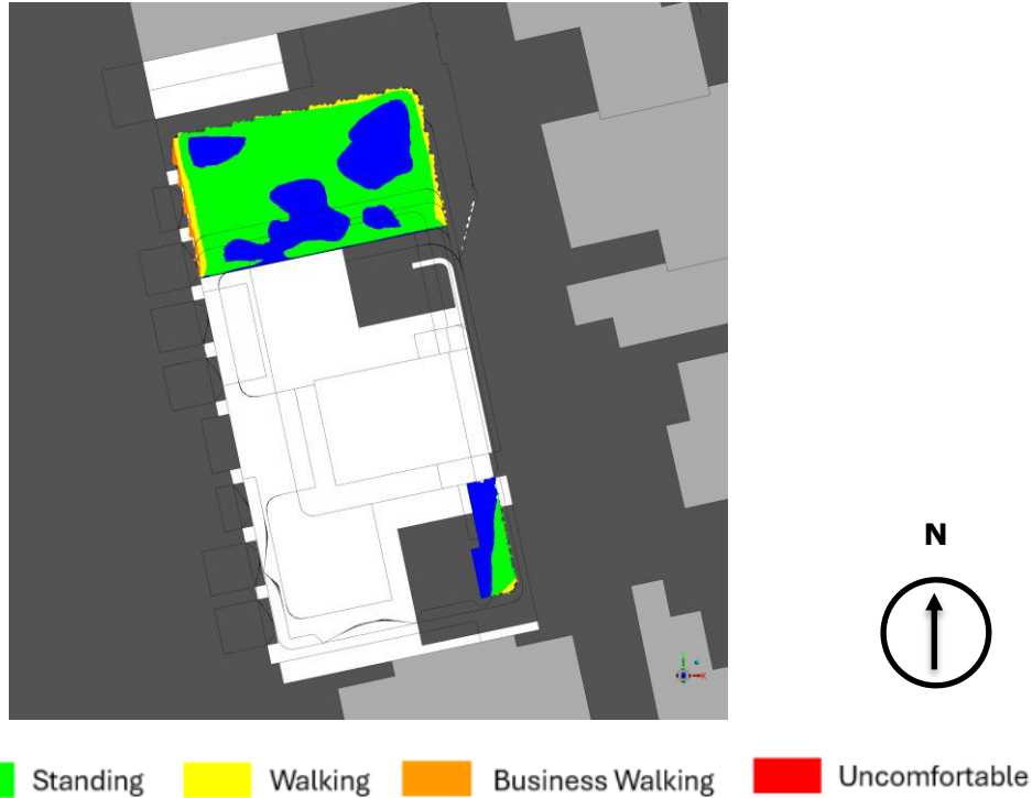
Figure 23: Wind comfort result (combined all wind directions) – level 11 terrace.
