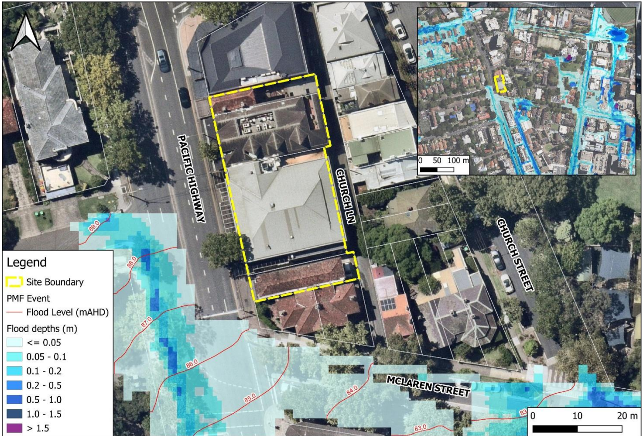
Figure 9: Flood levels and depths around the site area in the PMF event
