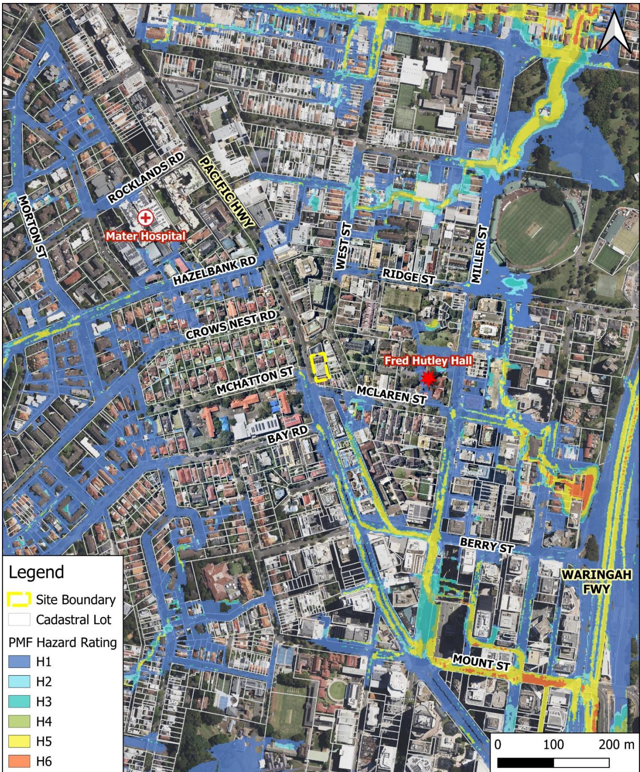
Figure 14: Peak flood hazard in the wider area in the PMF event.
