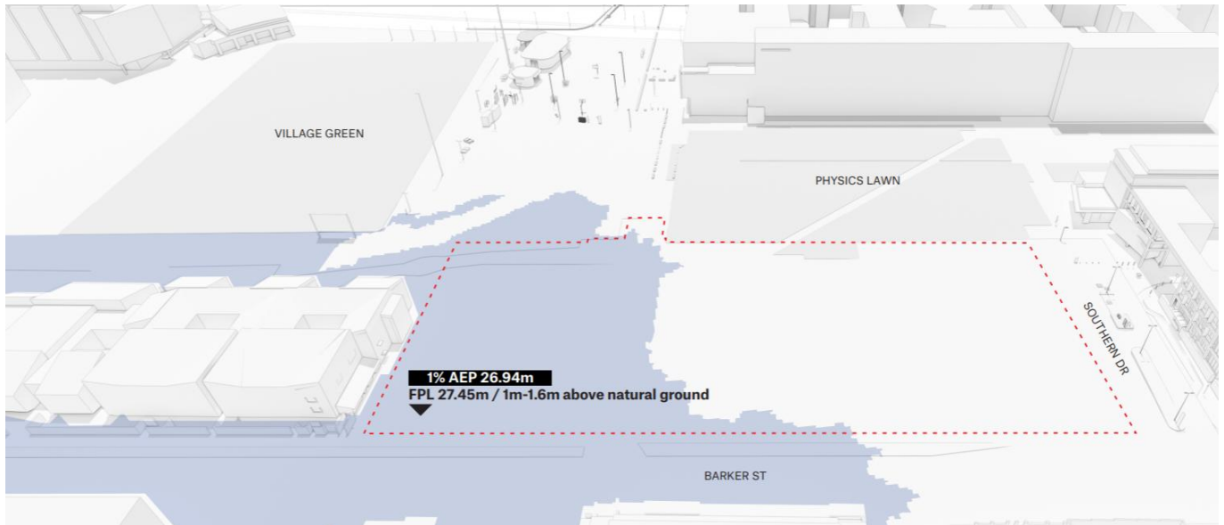
Figure 16 Portion of the site subject to flooding
