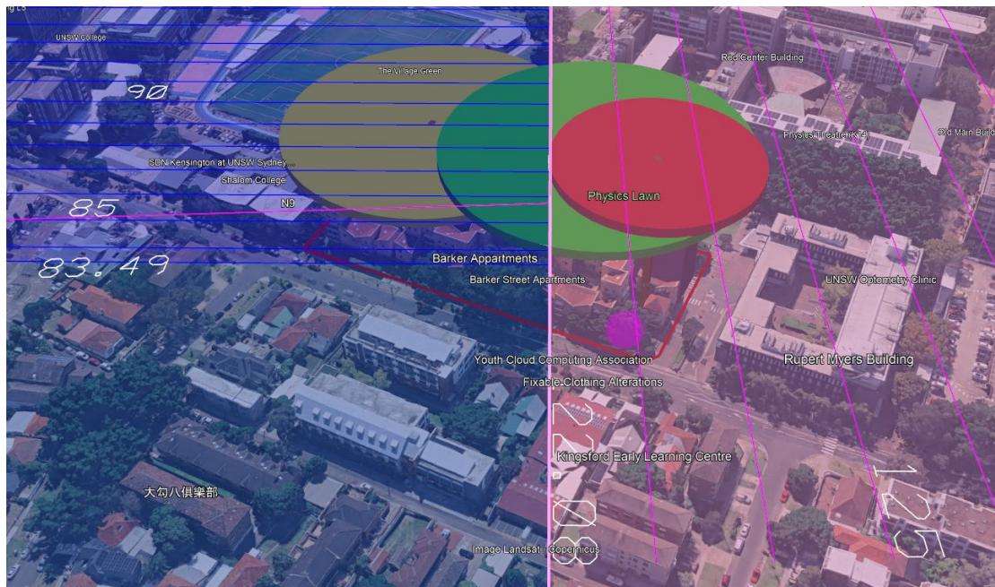
Figure 12: Avlaw's model of the PANS-OPS surfaces over the site (no intrusions proposed)
